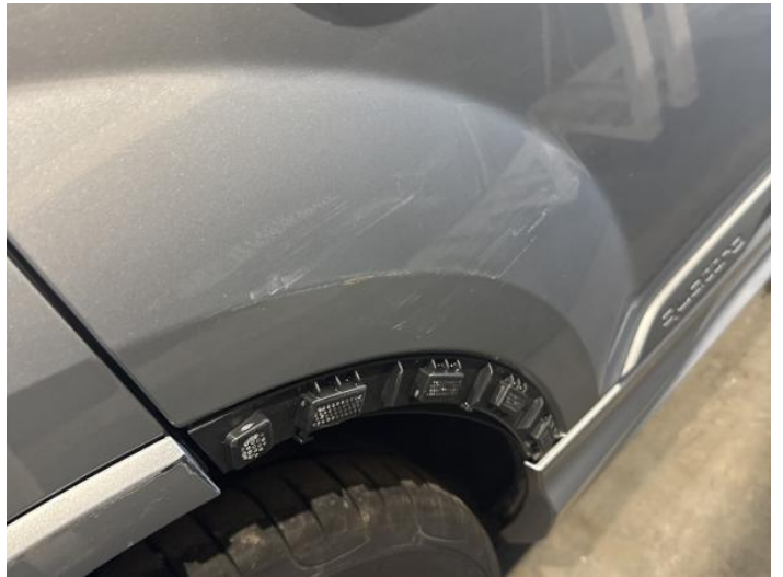
12: Door osr Dented With Paint Damage
