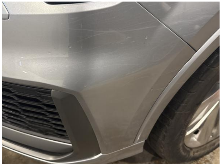
2: Bumper Front Scratched 25 to 100mm Thru Paint
