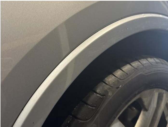
11: Qtr Panel Arch Extension os Scratched (Painted) Over 25mm Thru Paint
