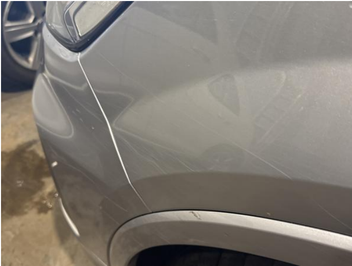
3: Wing nsf Scratched Over 25mm Thru Paint
