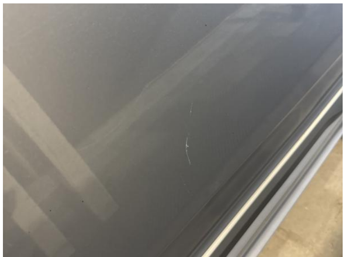
14: Door osf Scratched Over 25mm Thru Paint
