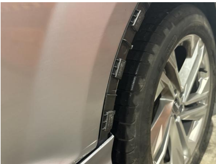
7: Door Moulding nsr Missing Replace
