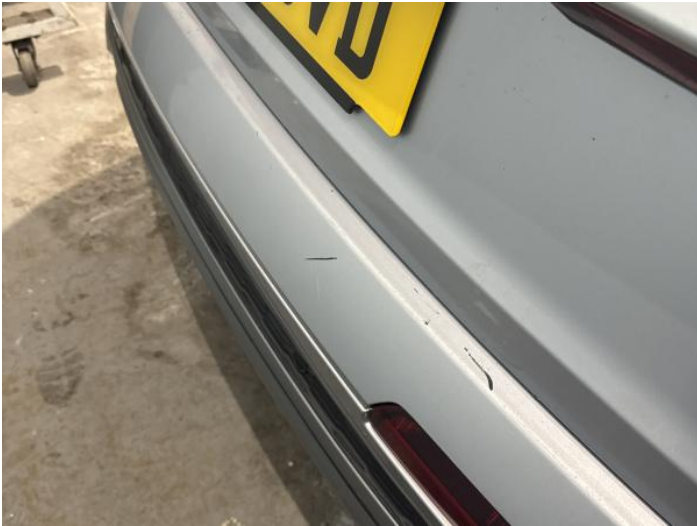
9: Bumper Rear Scratched Over 100mm Thru Paint
