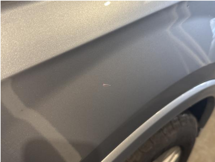
15: Wing of Scratched Up To 25mm Thru Paint
