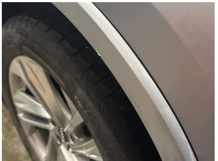
8: Qtr Panel Arch Extension ns Scratched (Painted) UpTo 25mm Thru Paint
