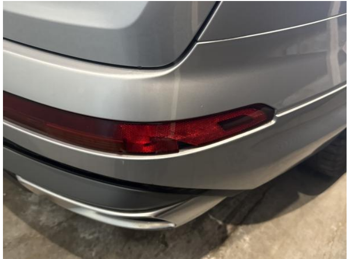
10: Bumper Reflector osr Broken Replace
