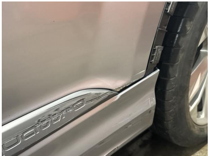
6: Door nsr Scratched Over 25mm Thru Paint
