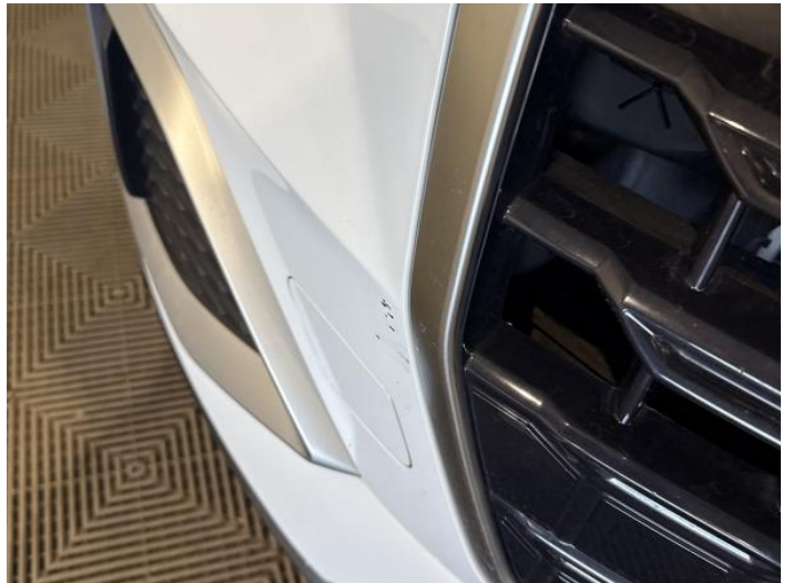
2: Bumper Front Scratched 25 to 100mm Thru Paint
