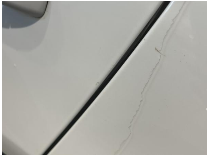
6: Door nsr Chipped 1 To 5
