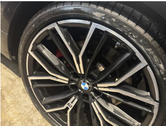
11: Wheel nsr Scratched Over 50mm
