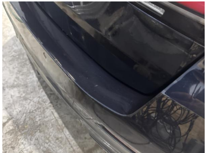
12: Bumper Rear Scratched 25 to 100mm Thru Paint
