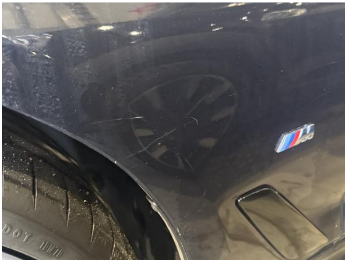
3: Wing nsf Scratched UpTo 25mm Thru Paint
