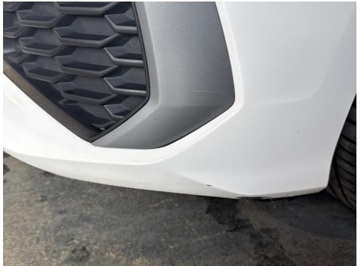
2: Bumper Front Scratched 25 to 100mm Thru Paint
