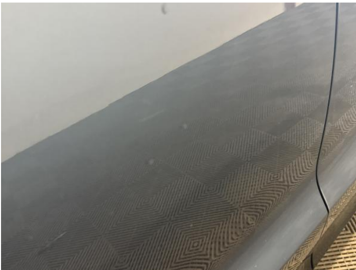
11: Door osr Scratched UpTo 25mm Thru Paint
