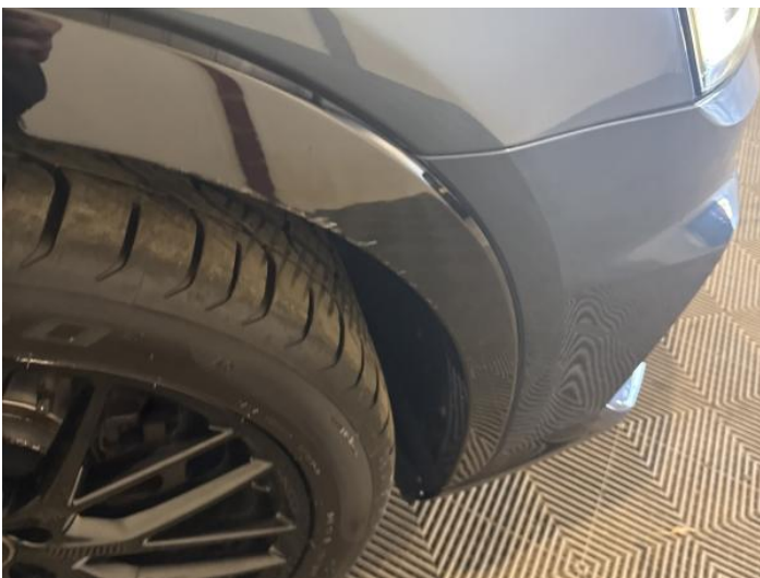
13: Wing Front Arch Extension os Scratched (Painted) Over 25mm Thru Paint
