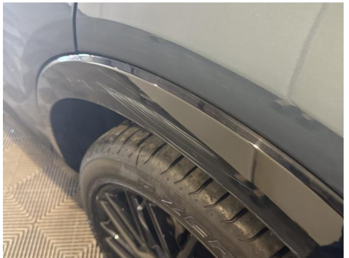
6: Qtr Panel Arch Extension ns Scratched (Painted) Over 25mm Thru Paint
