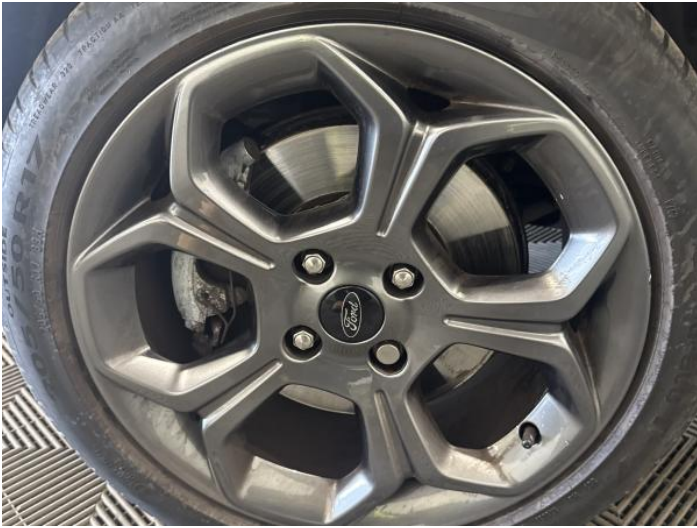
3: Wheel nsf Scratched Up To 50mm
