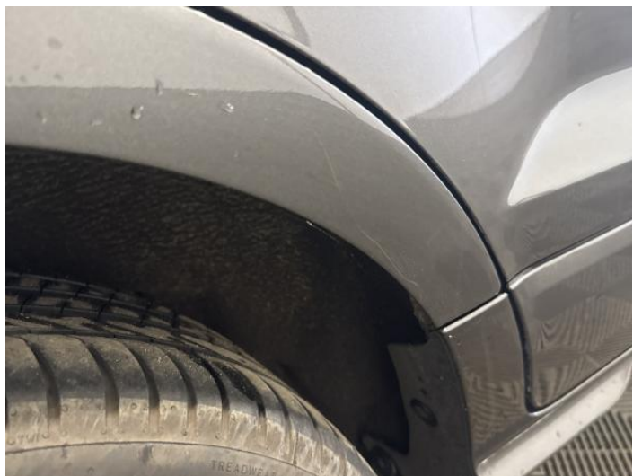
8: Qtr Panel osr Scratched Over 25mm Thru Paint
