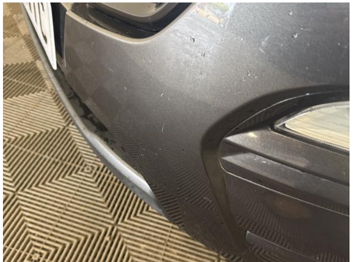
2: Bumper Front Chipped Multiple Chips
