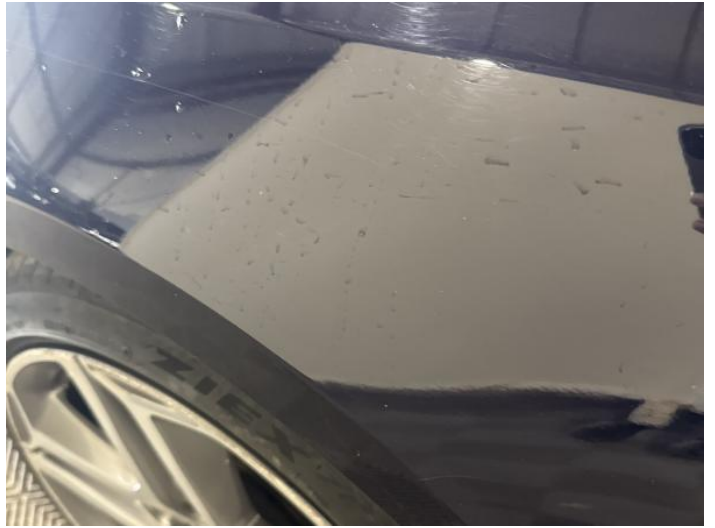
4: Wing nsf Scratched UpTo 25mm Thru Paint
