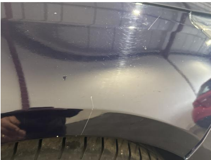
19: Wing osf Scratched Over 25mm Thru Paint
