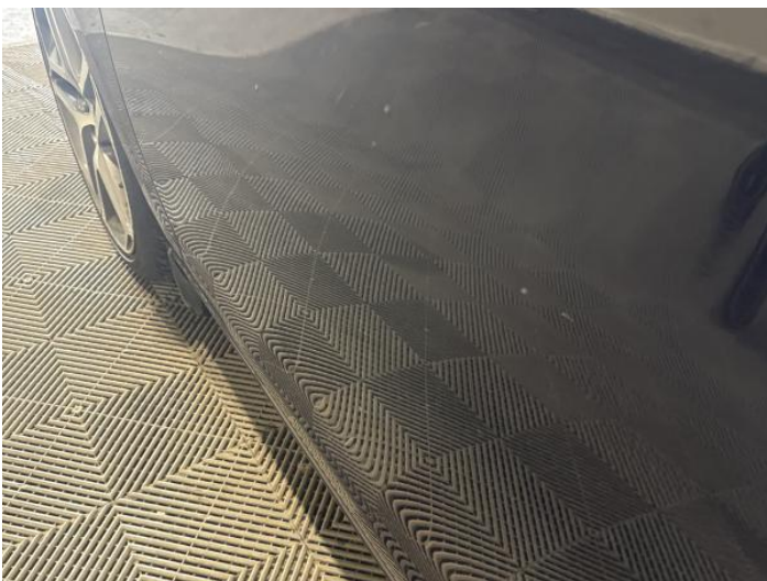
7: Door nsf Dented Between 10mm + 30mm
