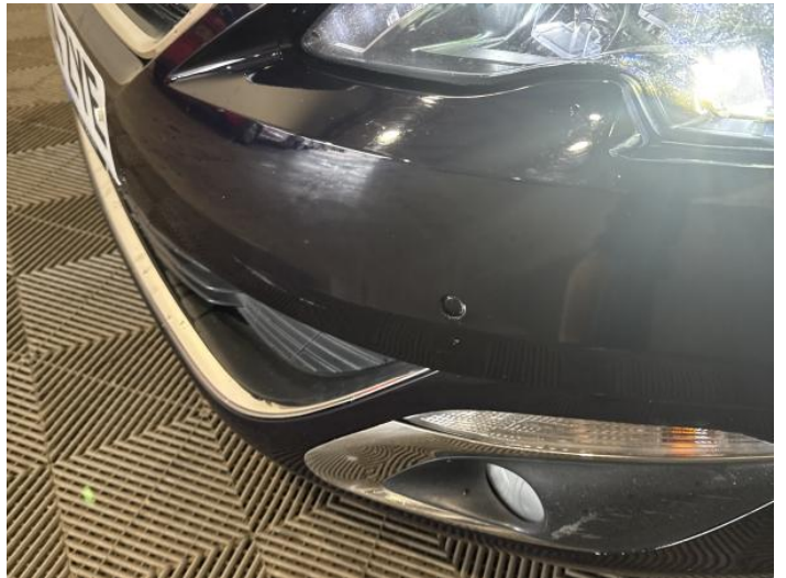
2: Bumper Front Scratched Over 100mm Thru Paint
