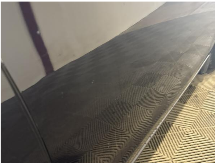
17: Door osf Dented With Paint Damage
