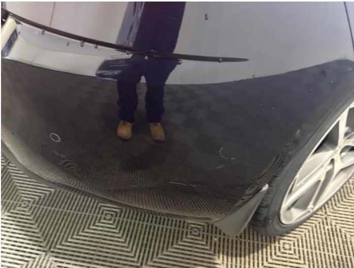
11: Bumper Rear Scratched Over 100mm Thru Paint
