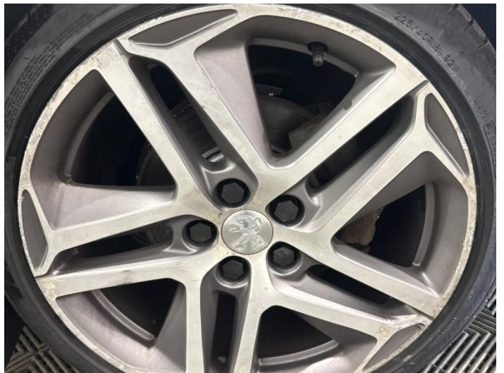
18: Wheel osf Scratched Over 50mm
