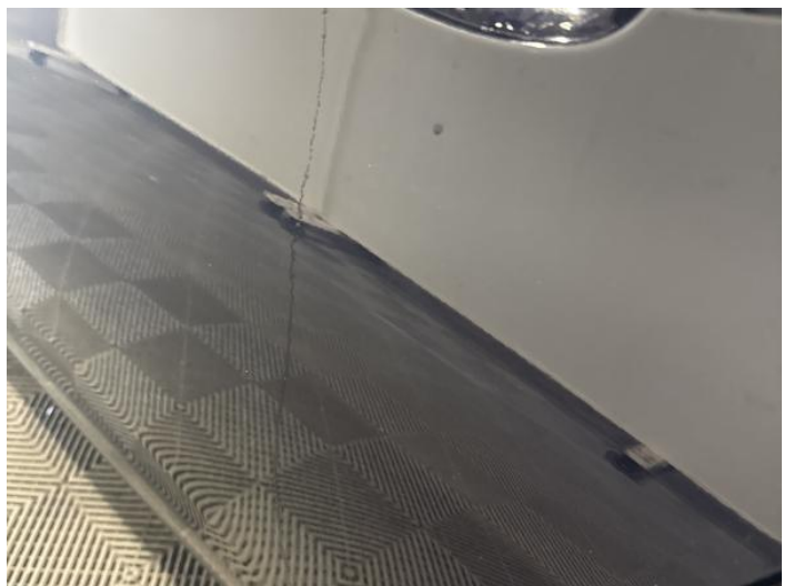
8: Door nsr Scratched Over 25mm Thru Paint
