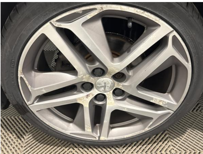
13: Wheel osr Scratched Over 50mm
