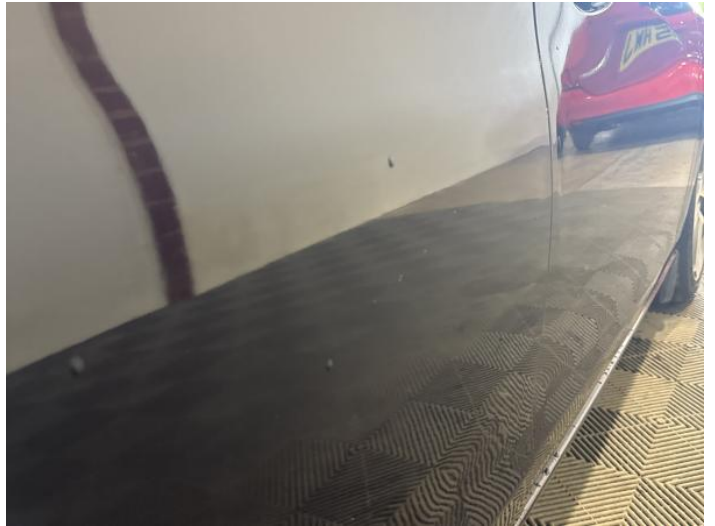
16: Door osr Poor Previous Repair Rippled Up To 30%
