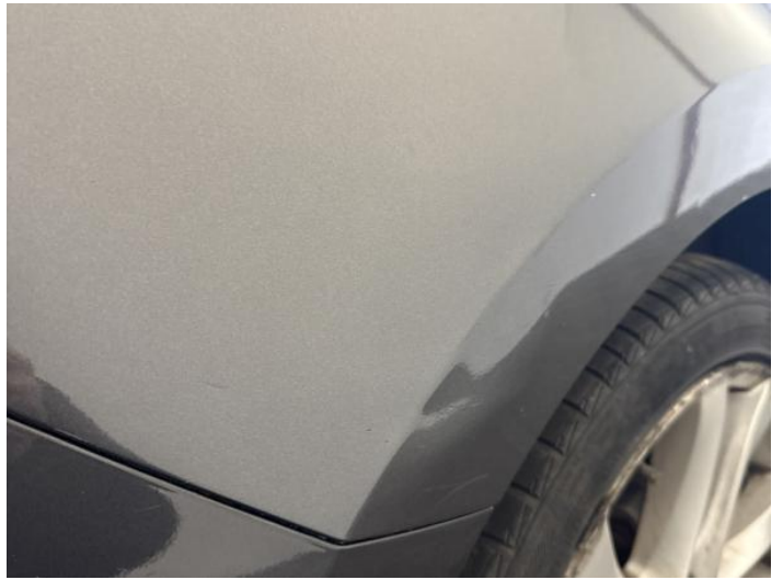
12: Qtr Panel osr Dented Over 30mm
