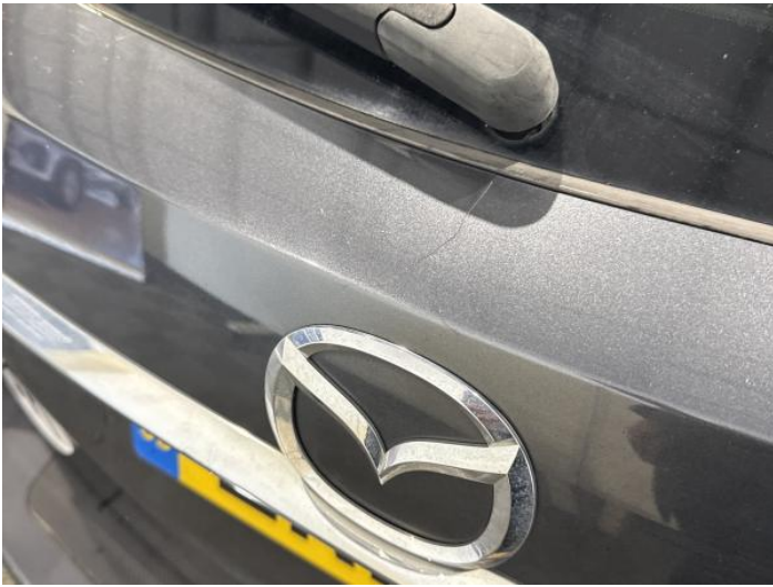
11: Tailgate Cracked Replace
