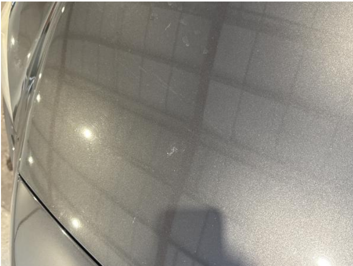
1: Bonnet Dented With Paint Damage
