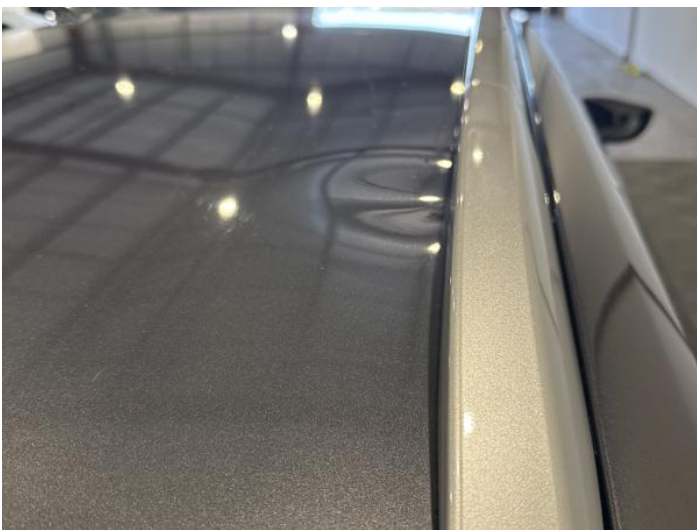
13: Roof Dented Over 30mm
