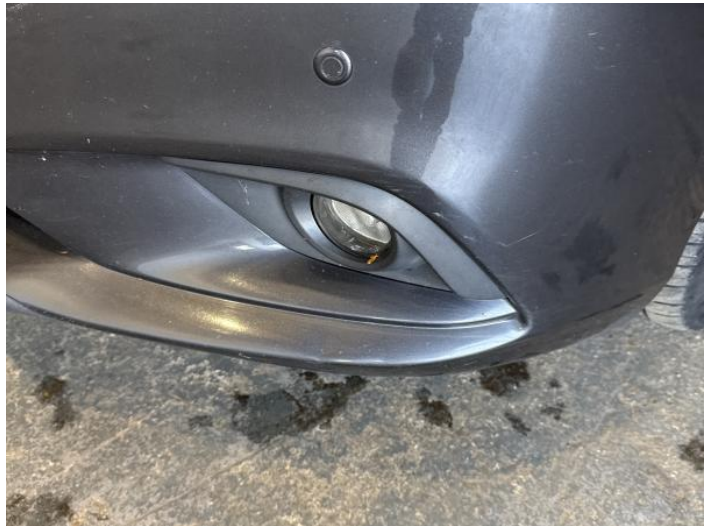
2: Bumper Front Dented With Paint Damage
