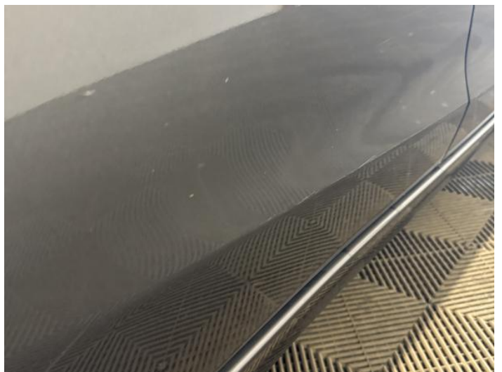
14: Door osr Dented With Paint Damage
