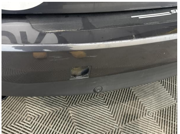
8: Rear TowEye Cvr Missing Replace
