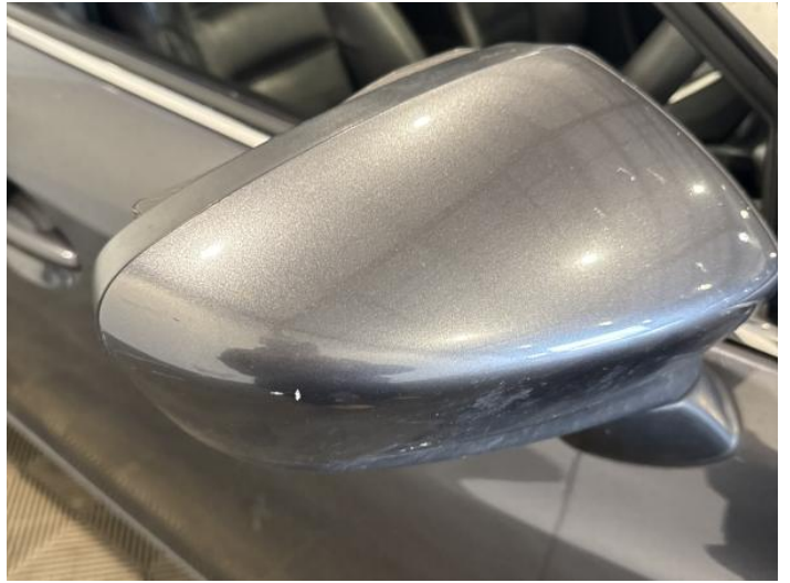
16: Door Mirror Assy osf Scratched (Painted) UpTo 25mm Thru Paint
