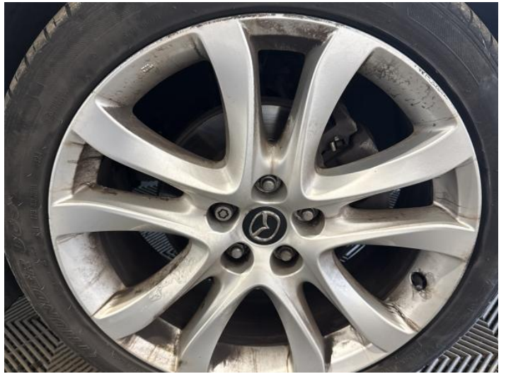
18: Wheel osf Scratched Over 50mm
