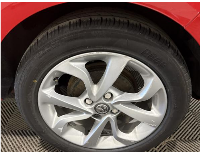
7: Wheel nsr Scratched Over 50mm
