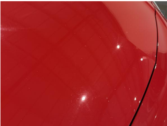
1: Bonnet Chipped Multiple Chips
