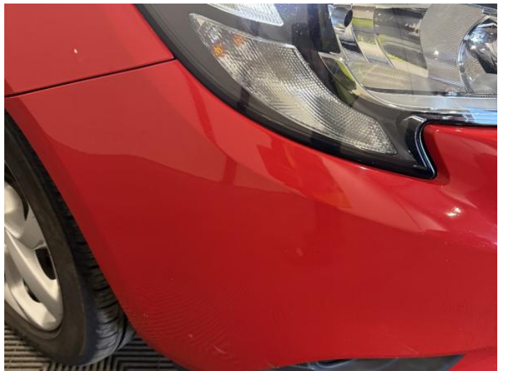
2: Bumper Front Scratched 25 to 100mm Thru Paint
