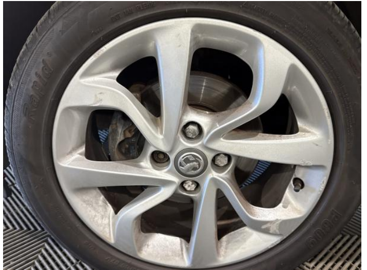
4: Wheel nsf Scratched Over 50mm
