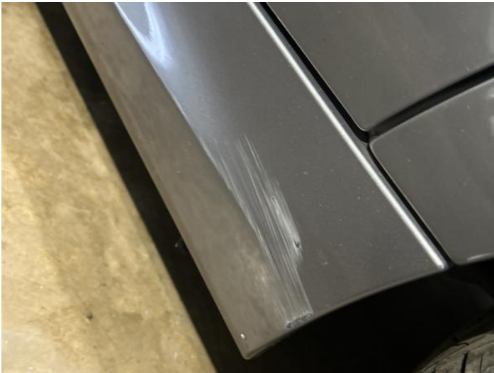
11: Sill Panel Trim ns Scratched (Painted) Over 25mm Thru Paint
