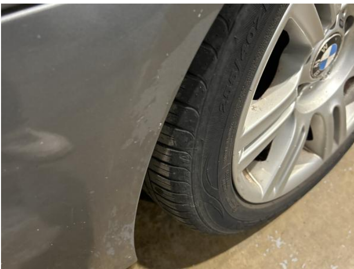
7: Bumper Rear Poor Previous Repair Paint Flake
