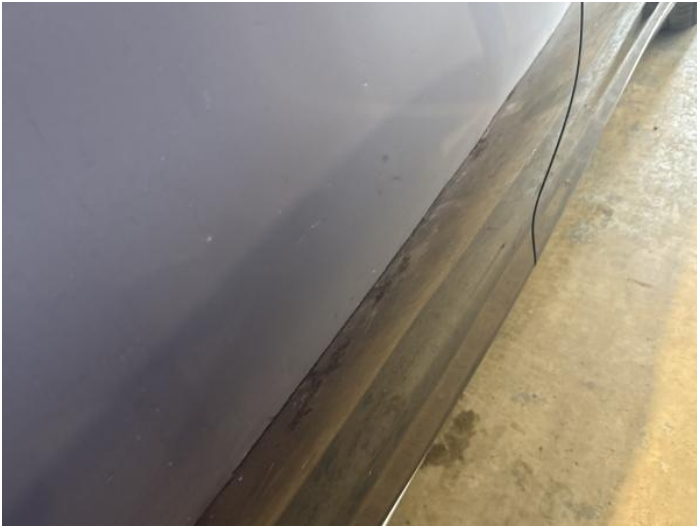
9: Door osr Dented Over 30mm
