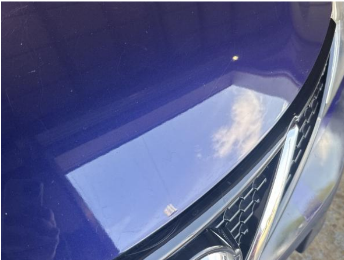
1: Bonnet Scratched Over 25mm Thru Paint
