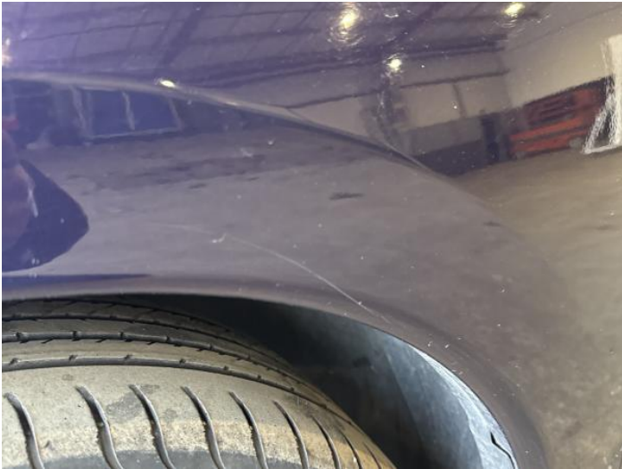
3: Wing nsf Scratched Over 25mm Thru Paint
