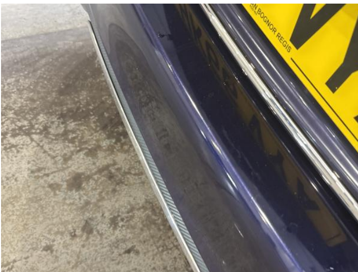
7: Bumper Rear Scratched 25 to 100mm Thru Paint
