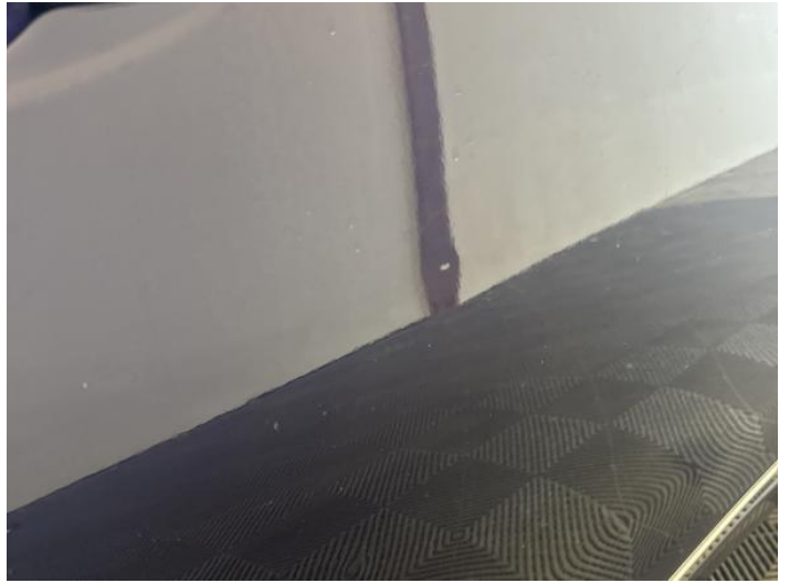
10: Door osf Dented Between 10mm + 30mm
