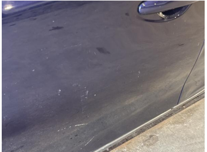
4: Door nsf Scratched Over 25mm Thru Paint
