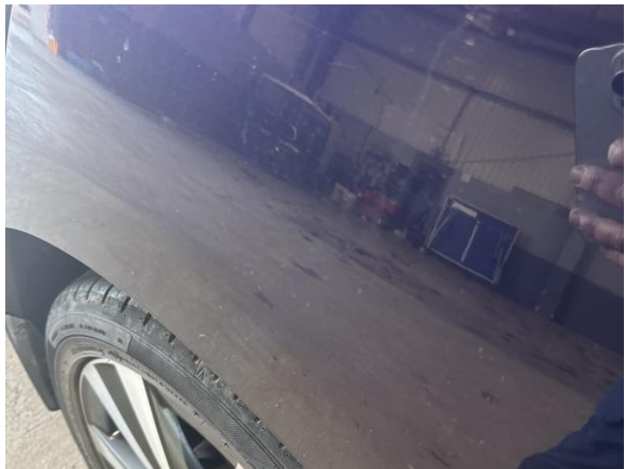
6: Qtr Panel nsr Scratched UpTo 25mm Thru Paint
