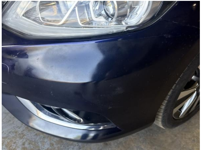
2: Bumper Front Poor Previous Repair Poor Paint
