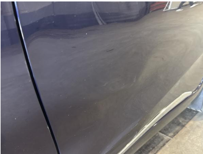
5: Door nsr Dented With Paint Damage
