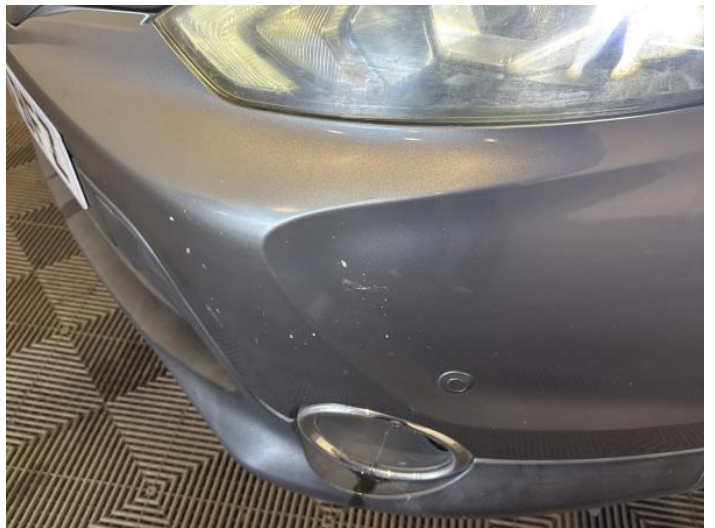
2: Bumper Front Poor Previous Repair Paint Flake
