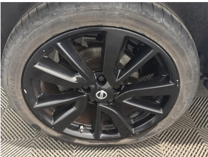
7: Wheel osr Scratched Over 50mm
