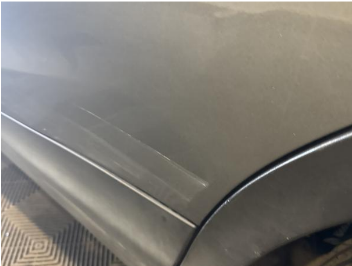
5: Door nsr Dented With Paint Damage
