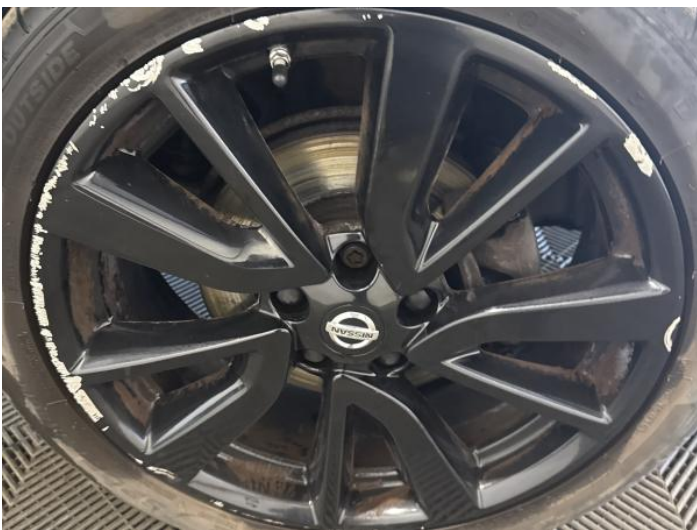
13: Wheel osf Scratched Over 50mm
