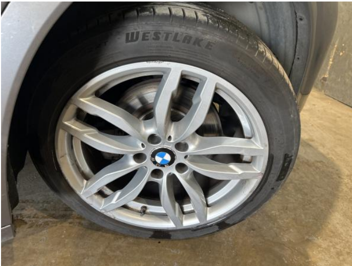
1: Wheel osf Scratched Over 50mm
