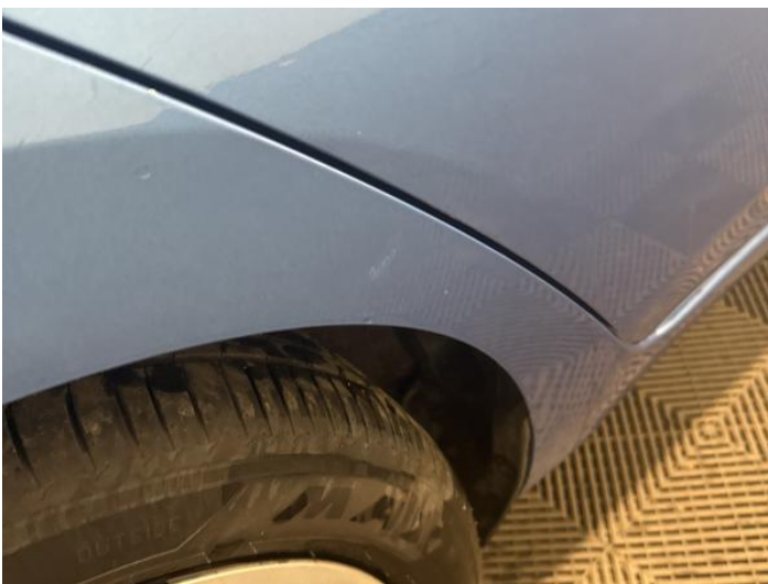
7: Qtr Panel osr Dented With Paint Damage
