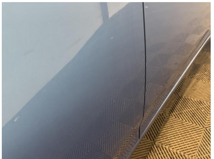
8: Door osr Scratched Over 25mm Thru Paint
