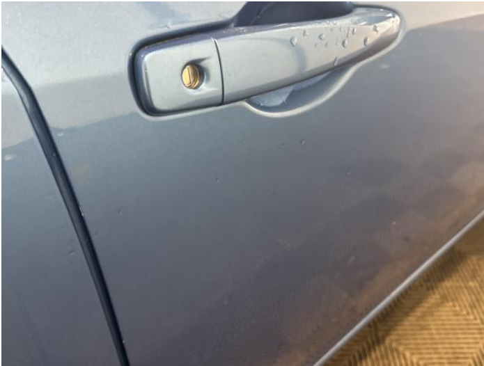
9: Door osf Scratched Over 25mm Thru Paint
