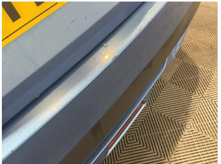
6: Bumper Rear Scratched 25 to 100mm Thru Paint
