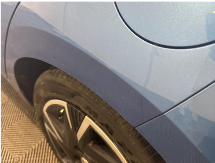
5: Qtr Panel nsr Scratched UpTo 25mm Thru Paint
