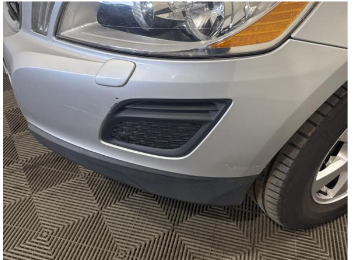
2: Bumper Front Scratched Over 100mm Thru Paint
