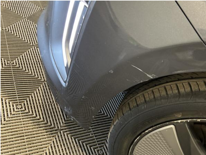
9: Bumper Front Scratched Over 100mm Thru Paint
