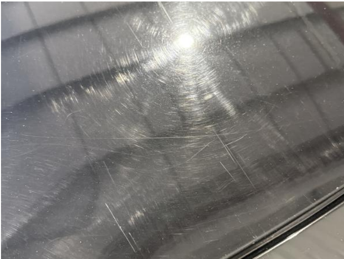
1: Bonnet Scratched Over 25mm Thru Paint
