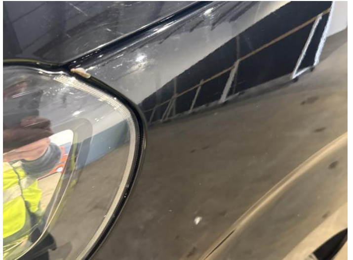
4: Wing nsf Scratched Over 25mm Thru Paint
