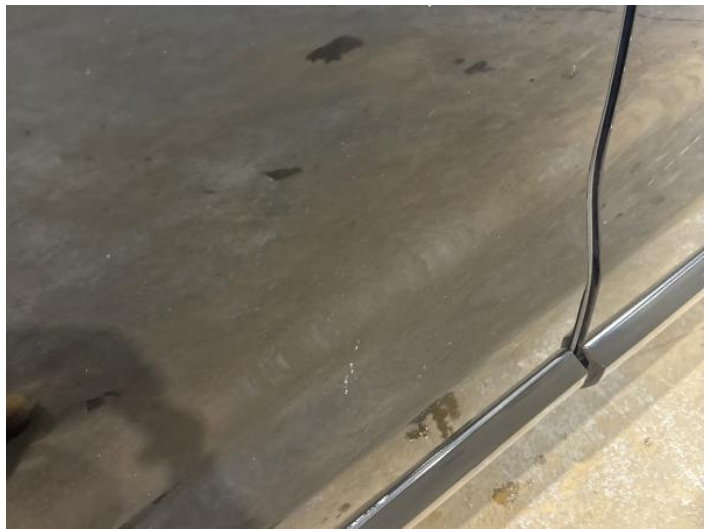
6: Door nsf Scratched Over 25mm Thru Paint
