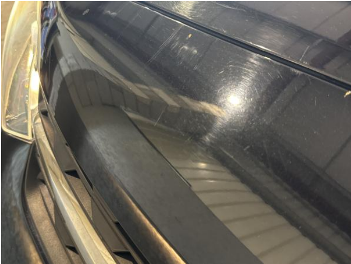
3: Bumper Front Moulding Scratched (Painted) Over 25mm Thru Paint
