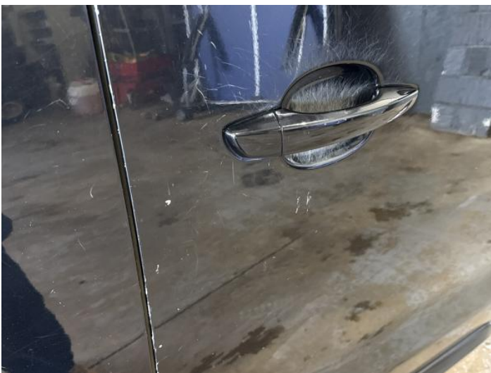
13: Door osf Scratched Over 25mm Thru Paint
