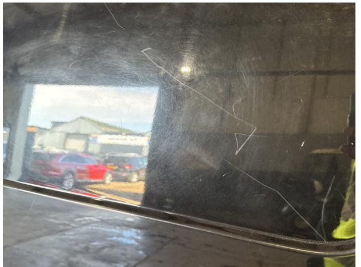
12: Door osr Scratched Over 25mm Thru Paint
