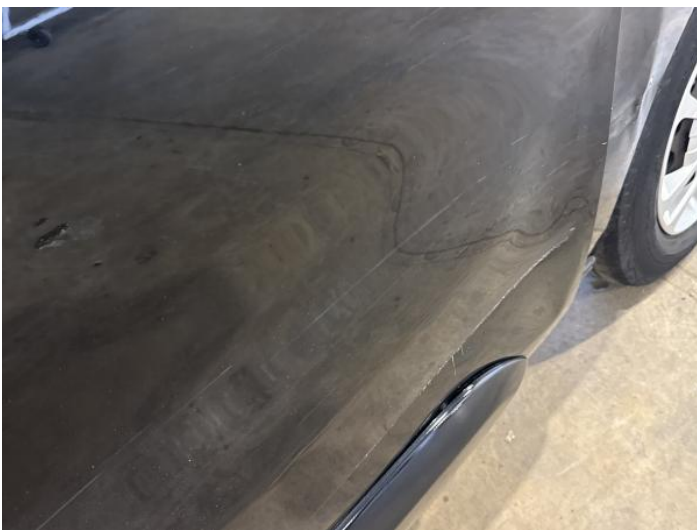
7: Door nsr Dented With Paint Damage
