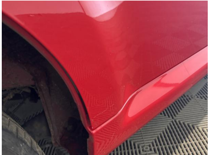
10: Door osf Scratched Over 25mm Thru Paint
