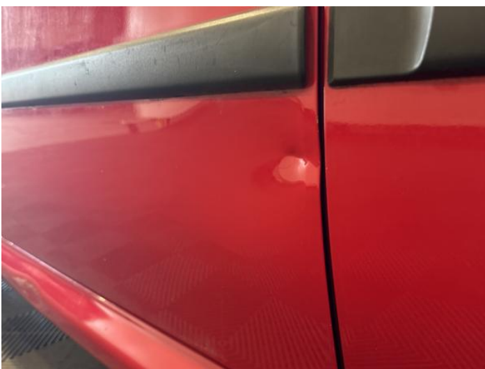
7: Door nsf Dented With Paint Damage
