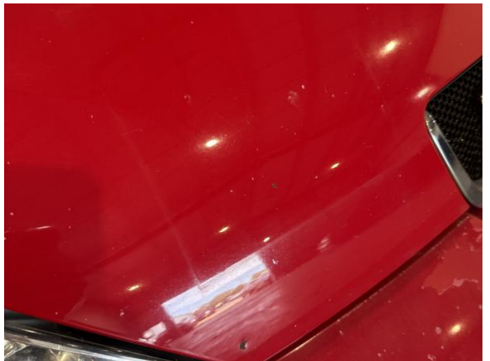
2: Bonnet Dented With Paint Damage
