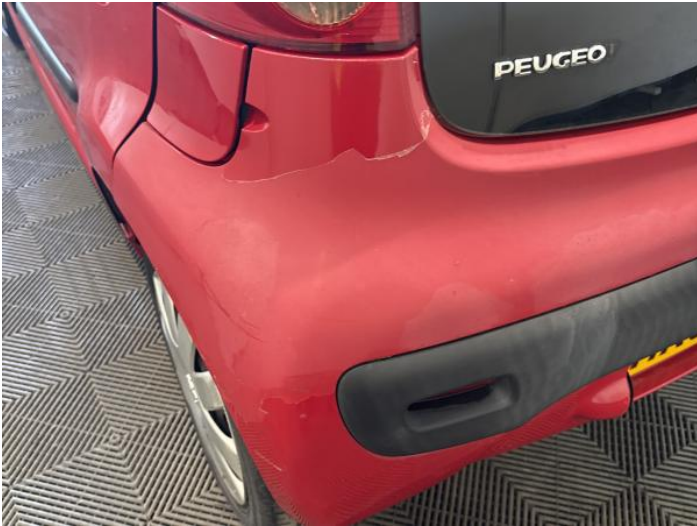
9: Bumper Rear Poor Previous Repair Paint Flake
