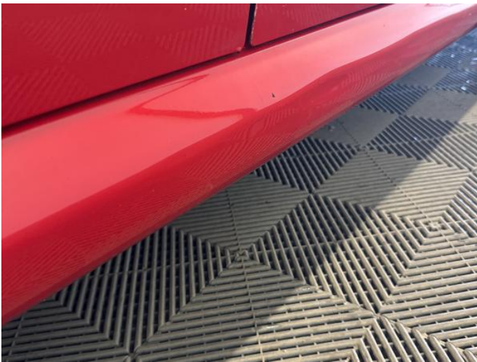
11: Sill os Dented Over 30mm
