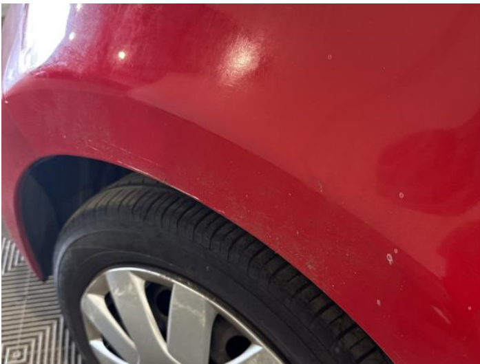
5: Wing nsf Scratched Over 25mm Thru Paint
