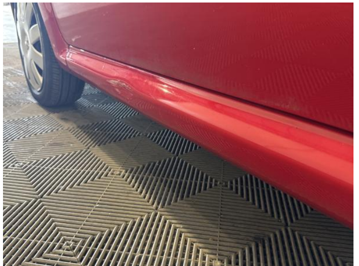
6: Sill ns Dented With Paint Damage
