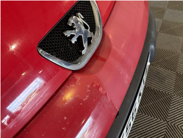
3: Bumper Front Poor Previous Repair Paint Flake
