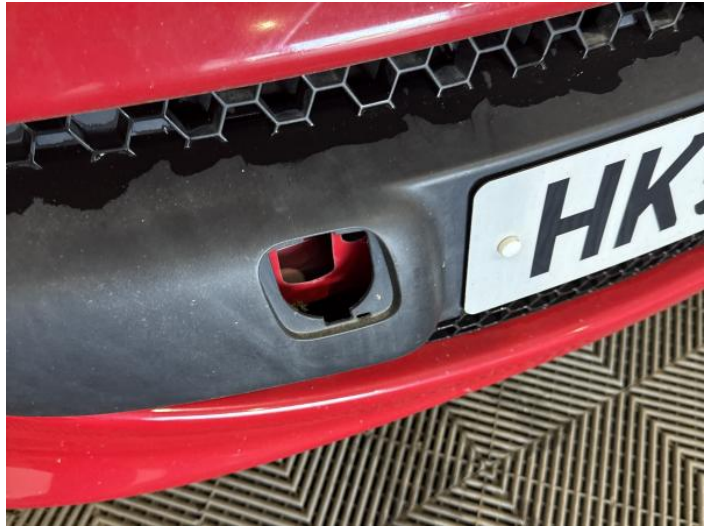
4: Front TowEye Cvr Missing Replace
