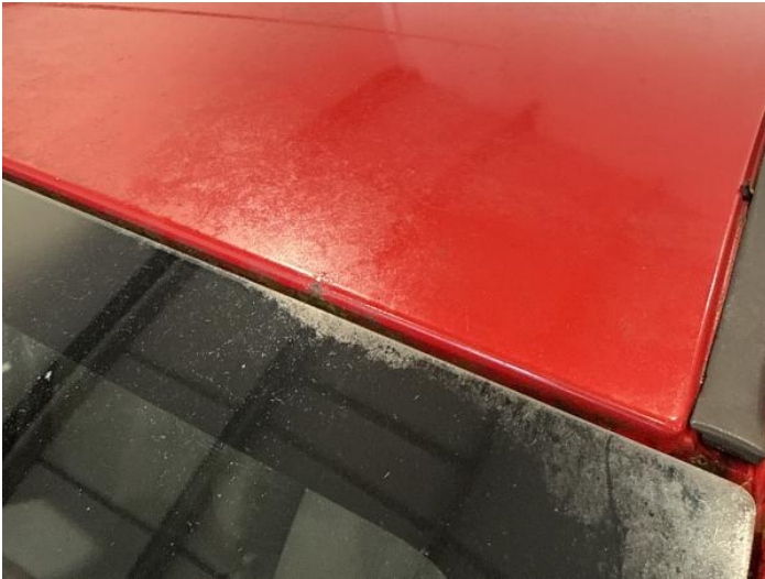
15: Roof Chipped Edge Chip
