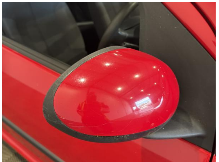
14: Door Mirror Assy osf Scratched (Painted) Over 25mm Thru Paint
