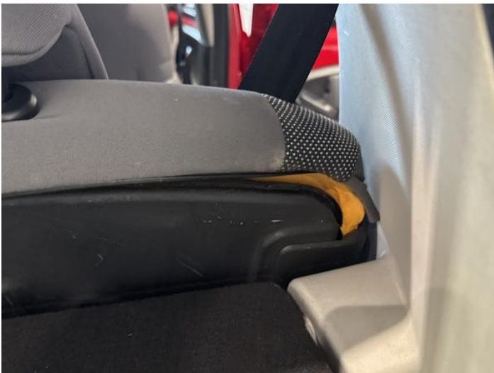
1: Seat Back Cover osr Torn Over 3mm
