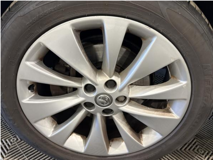
3: Wheel nsf Scratched Over 50mm
