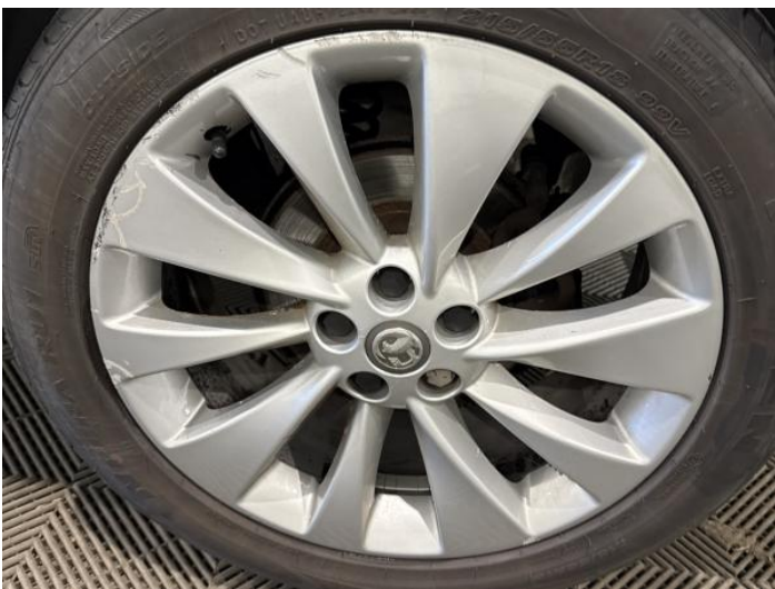
7: Wheel nsr Scratched Over 50mm
