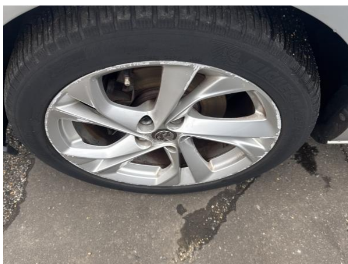
8: Wheel nsf Scratched Over 50mm
