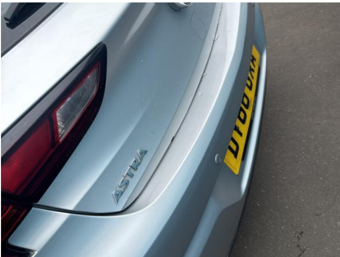
1: Bumper Rear Scratched 25 to 100mm Thru Paint
