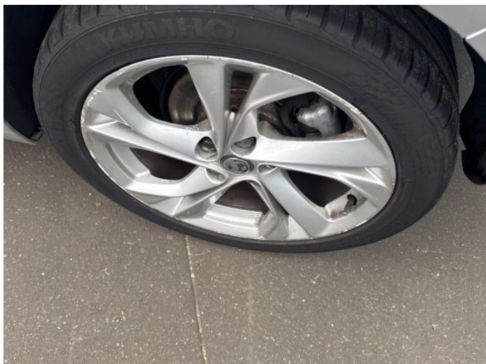
3: Wheel nsr Scratched Over 50mm
