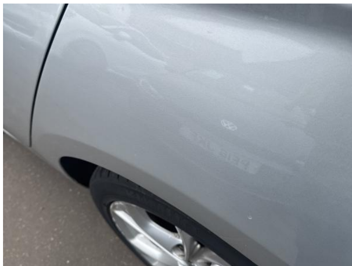
4: Qtr Panel nsr Dented Over 2 UpTo 10mm
