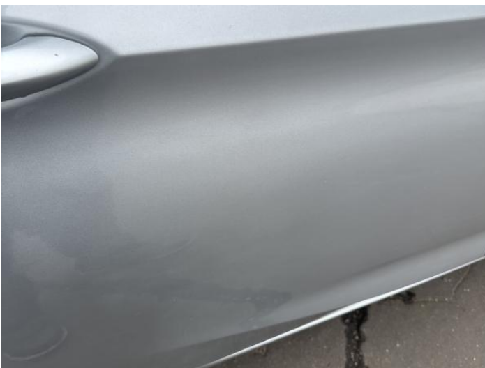
13: Door osr Poor Previous Repair Poor Paint
