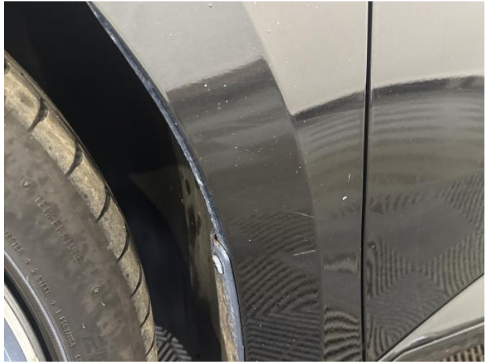
4: Wing nsf Scratched Over 25mm Thru Paint
