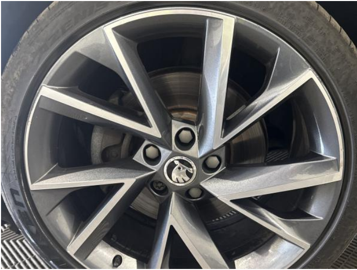
3: Wheel nsf Scratched Over 50mm
