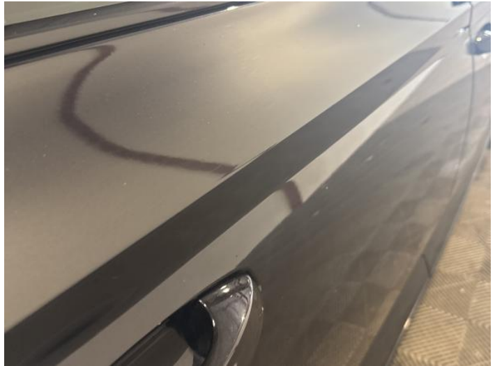
16: Door osr Dented Between 10mm + 30mm
