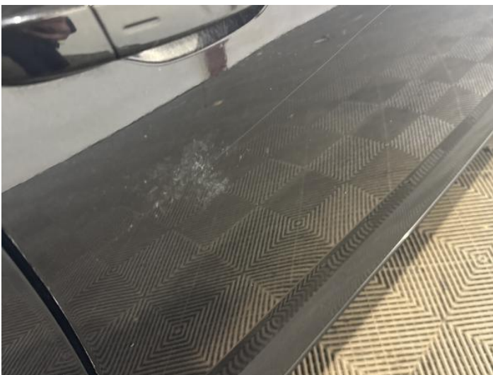
13: Door osf Scratched Over 25mm Thru Paint
