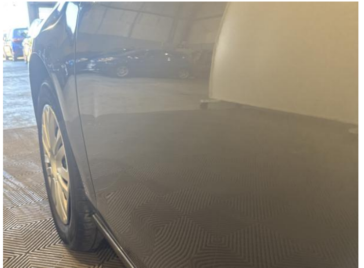
6: Door nsf Dented With Paint Damage
