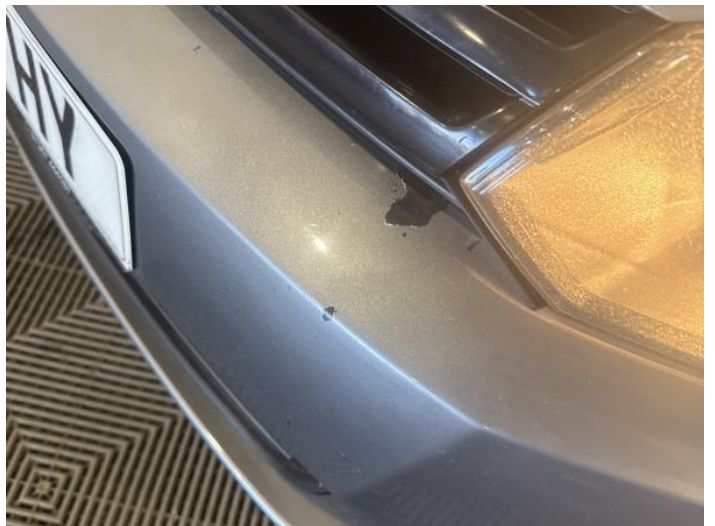
2: Bumper Front Poor Previous Repair Paint Flake
