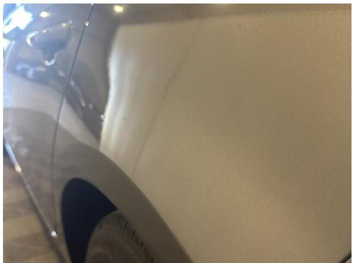
8: Qtr Panel nsr Poor Previous Repair Poor Paint
