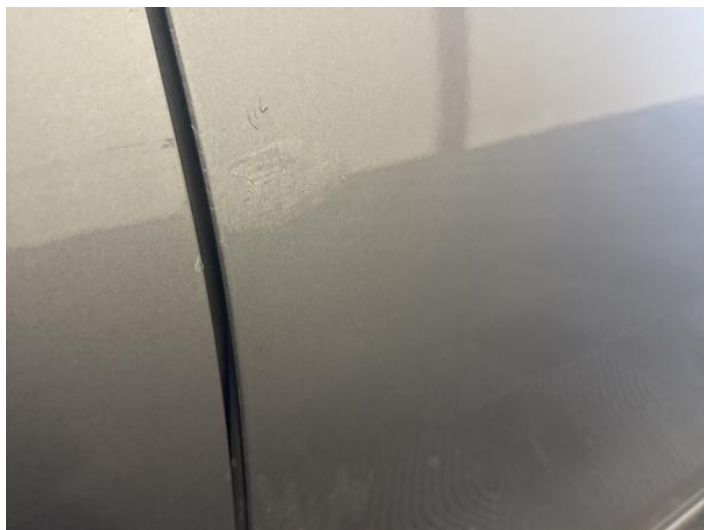
14: Door osf Scratched Over 25mm Thru Paint
