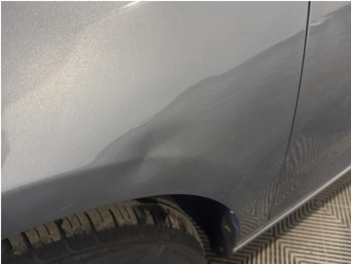
3: Wing nsf Dented Over 30mm
