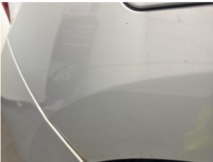
13: Qtr Panel osr Scratched Over 25mm Thru Paint
