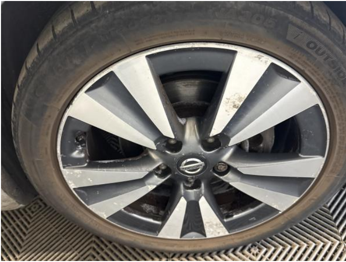
15: Wheel of Scratched Over 50mm
