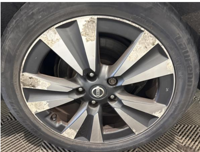
7: Wheel nsr Scratched Over 50mm
