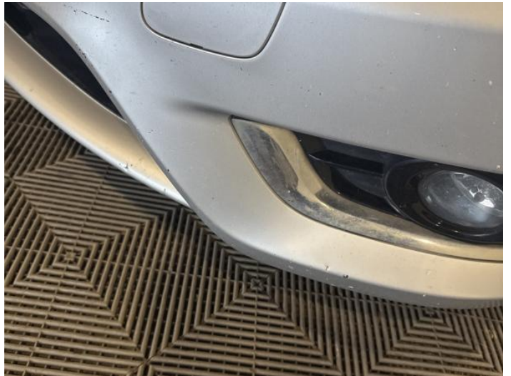
2: Bumper Front Dented With Paint Damage
