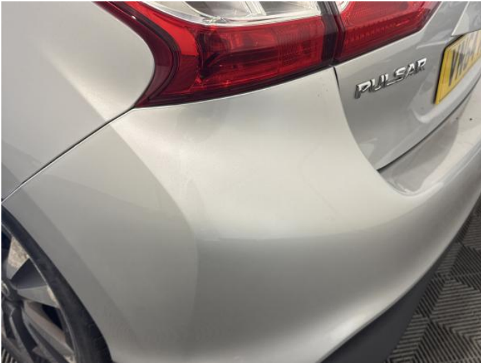
9: Bumper Rear Scratched 25 to 100mm Thru Paint
