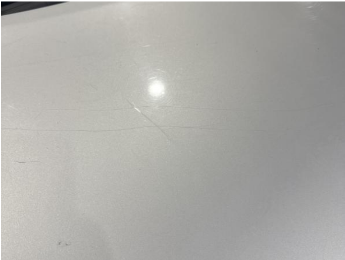
1: Bonnet Scratched Over 25mm Thru Paint
