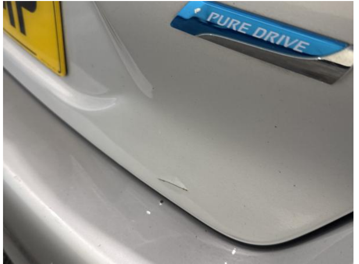
10: Tailgate Dented With Paint Damage
