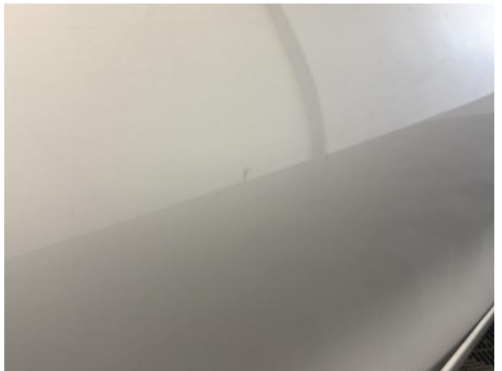
12: Door osr Dented With Paint Damage
