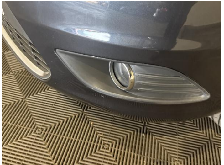
2: Bumper Front Scratched 25 to 100mm Thru Paint
