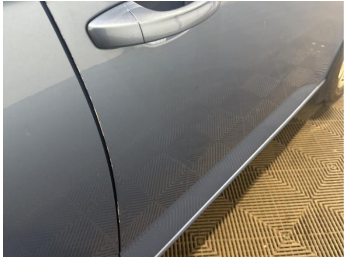
16: Door osf Dented With Paint Damage
