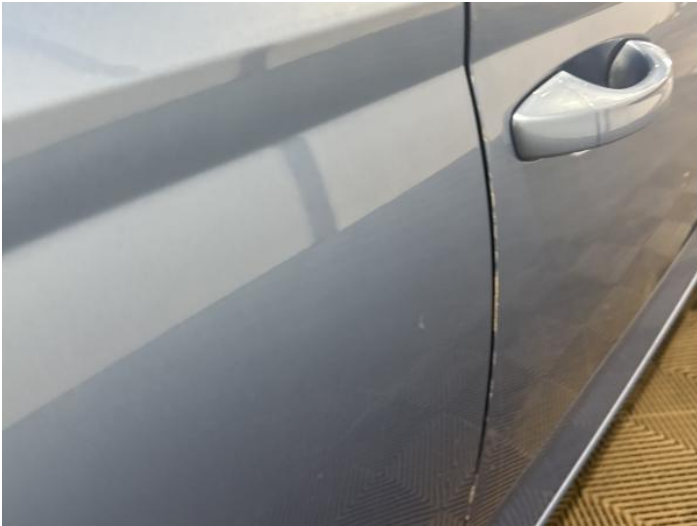
15: Door osr Dented Between 10mm + 30mm
