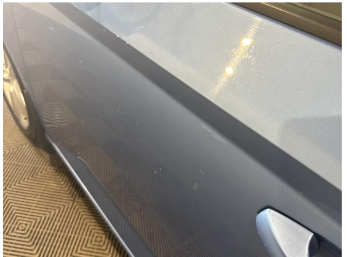
6: Door nsf Dented With Paint Damage
