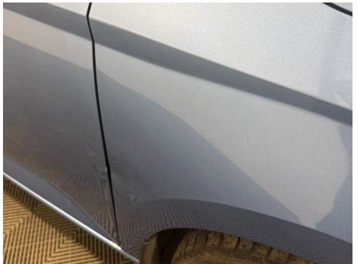
18: Wing nsf Dented Over 30mm
