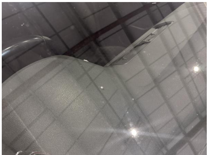
20: Screen Front Chipped UpTo 10mm
