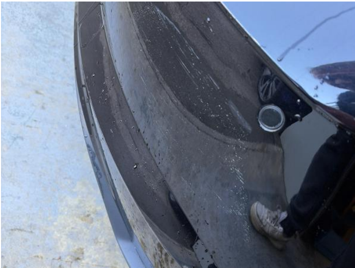
5: Bumper Rear Scratched 25 to 100mm Thru Paint
