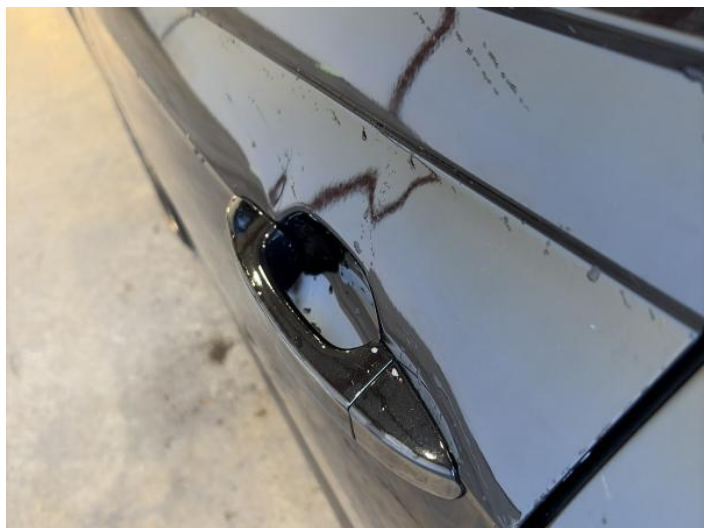
8: Door nsf Dented Over 30mm
