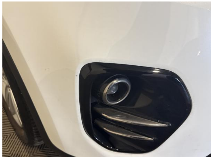
2: Bumper Front Scratched 25 to 100mm Thru Paint
