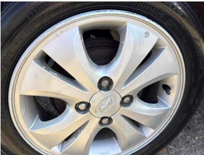
11: Wheel osr Scratched Over 50mm
