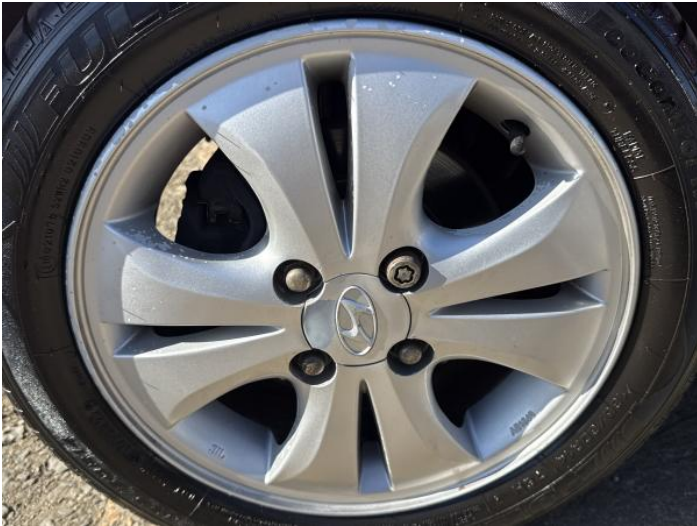
3: Wheel nsf Scratched Over 50mm
