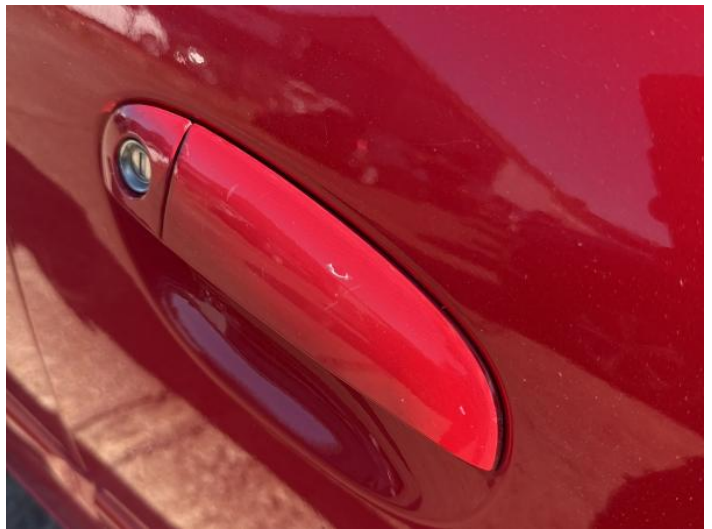
12: Door osf Scratched UpTo 25mm Thru Paint
