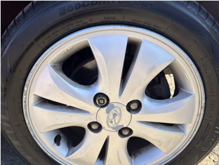
15: Wheel of Scratched Over 50mm
