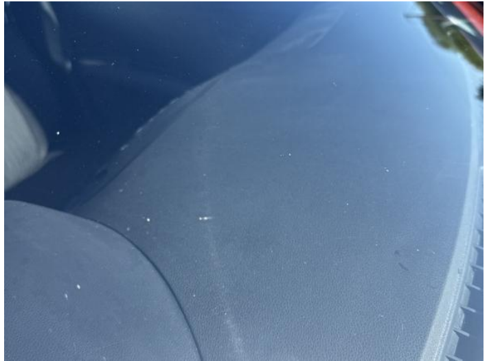
16: Screen Front Chipped UpTo 10mm
