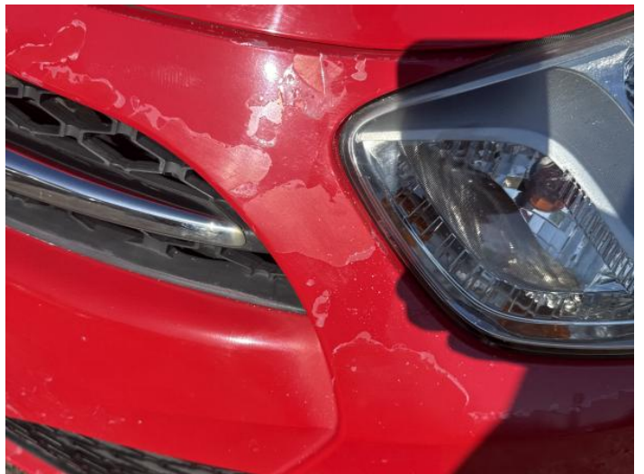
2: Bumper Front Poor Previous Repair Paint Flake
