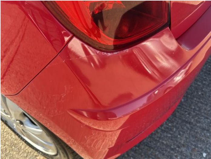
9: Bumper Rear Poor Previous Repair Paint Flake
