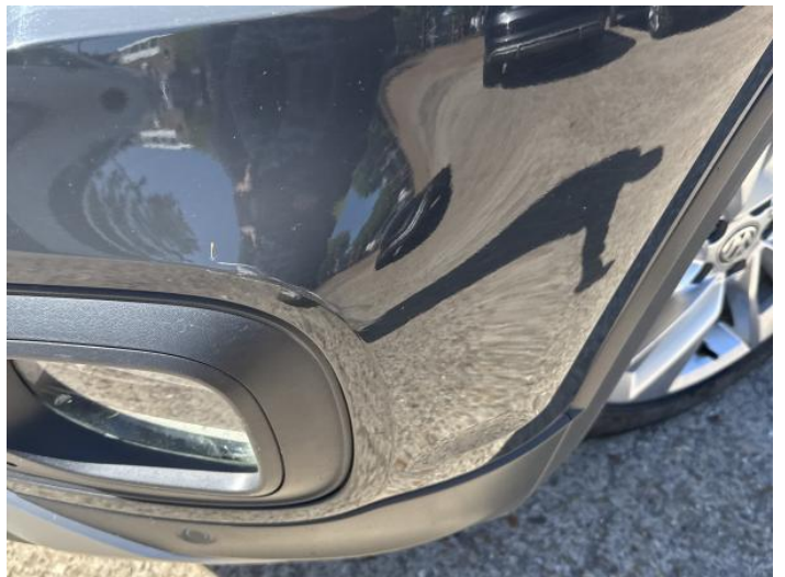
2: Bumper Front Scratched 25 to 100mm Thru Paint
