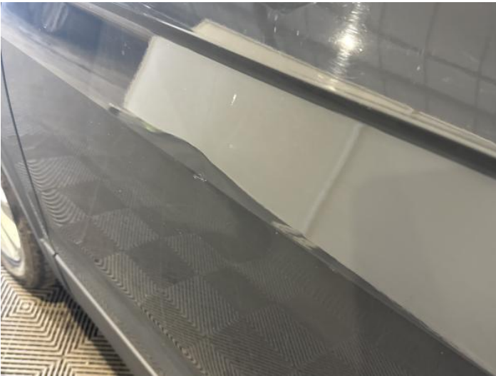
5: Door nsf Dented With Paint Damage
