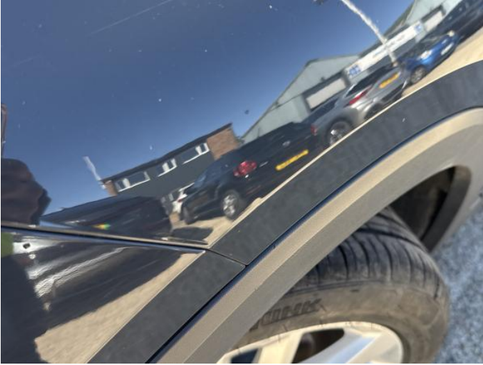
3: Wing nsf Dented Between 10mm + 30mm
