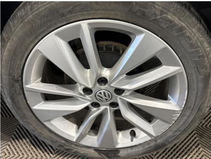
7: Wheel nsr Scratched Over 50mm
