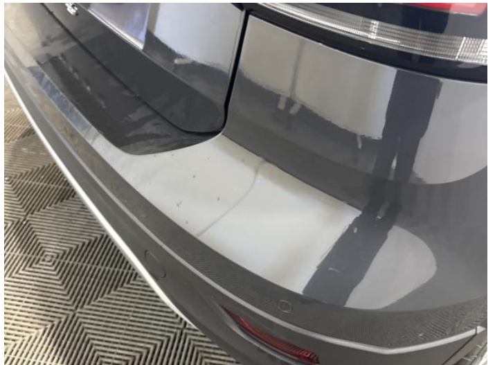
8: Bumper Rear Scratched 25 to 100mm Thru Paint
