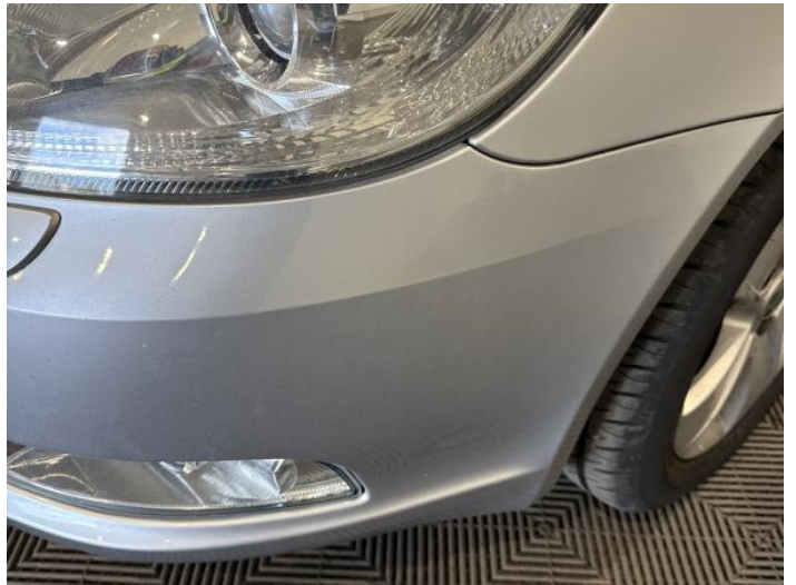
2: Bumper Front Scratched 25 to 100mm Thru Paint
