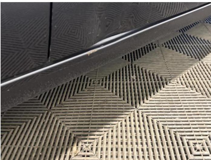
13: Sill os Scratched Over 25mm Thru Paint
