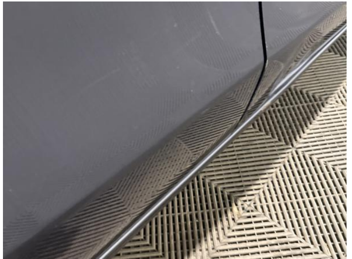
12: Door osr Scratched Over 25mm Thru Paint
