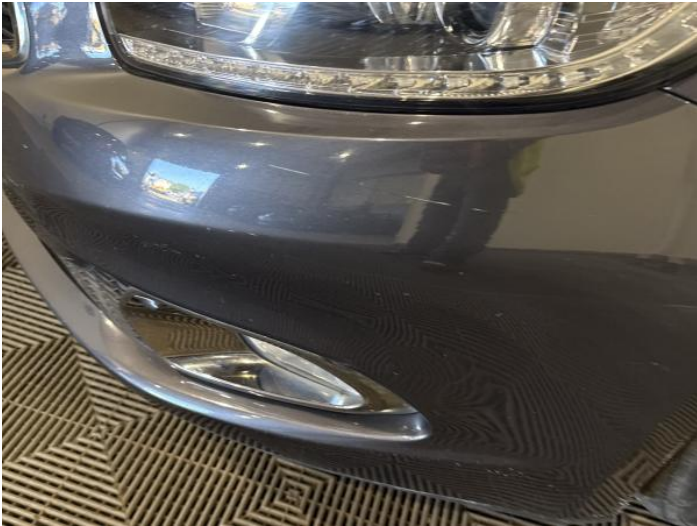
3: Bumper Front Scratched Over 100mm Thru Paint
