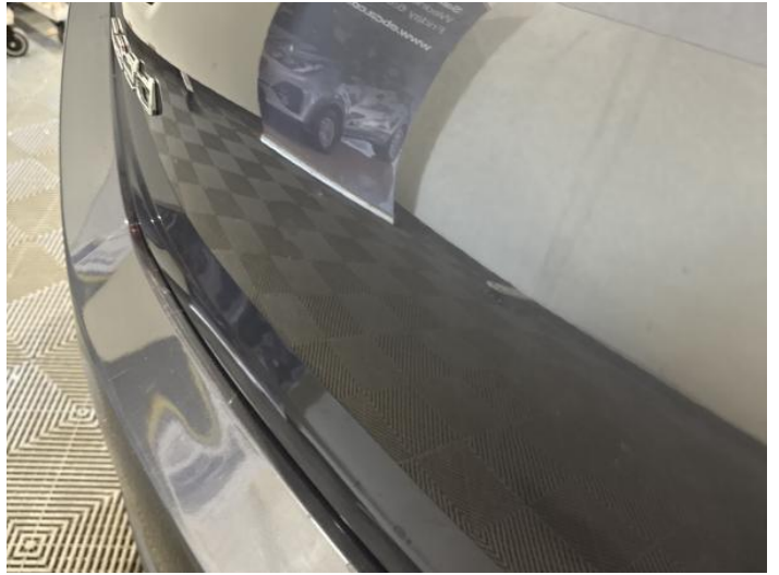
10: Tailgate Dented Between 10mm + 30mm
