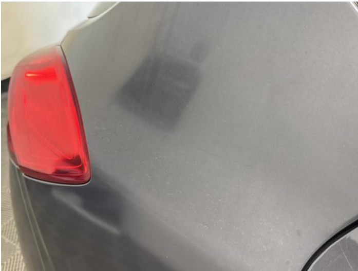
11: Qtr Panel osr Poor Previous Repair Poor Paint
