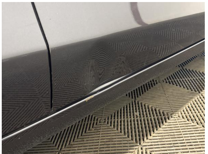
14: Door osf Dented Over 30mm
