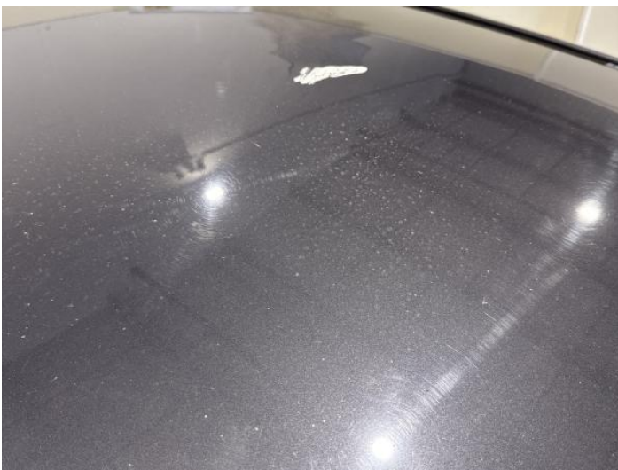
19: Roof Scratched Over 25mm Thru Paint
