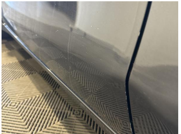
6: Door nsf Dented Over 30mm
