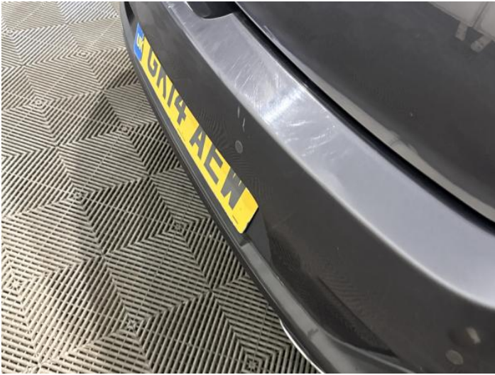
9: Bumper Rear Scratched 25 to 100mm Thru Paint
