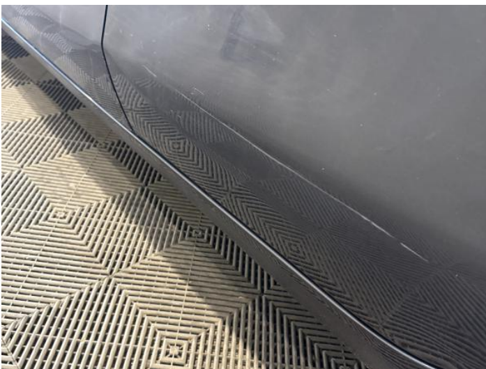
7: Door nsr Dented With Paint Damage
