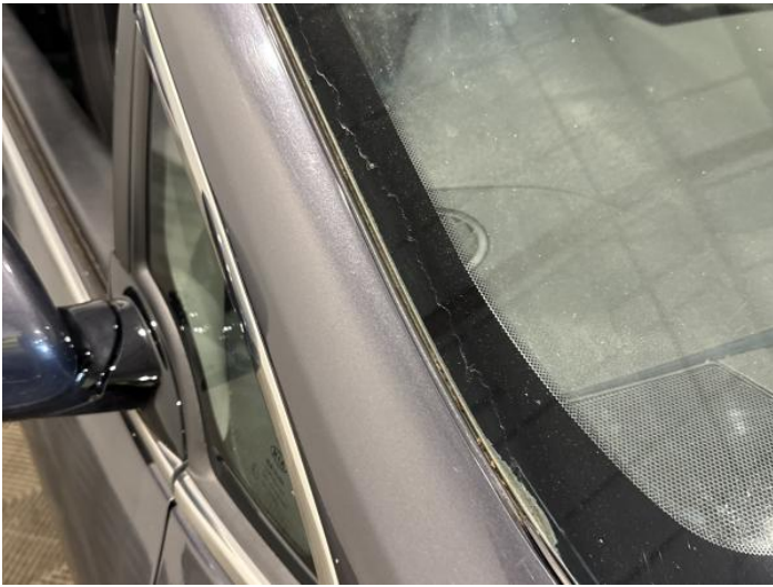
17: A Post os Scratched Over 25mm Thru Paint
