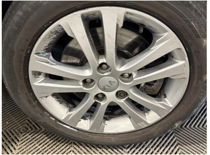
16: Wheel osf Scratched Over 50mm
