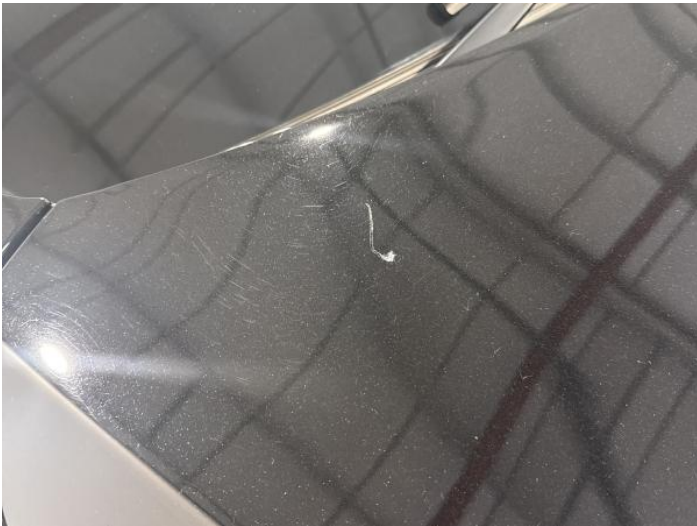
1: Bonnet Scratched Over 25mm Thru Paint
