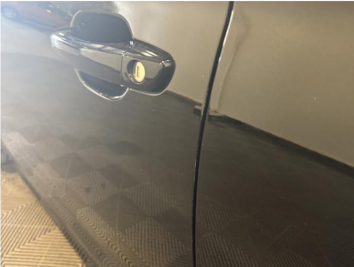
3: Door nsf Chipped Edge Chip
