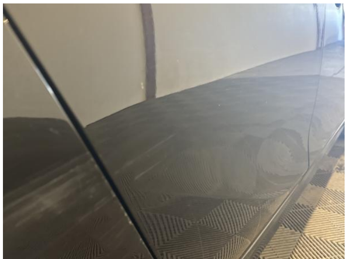
8: Door osr Dented With Paint Damage
