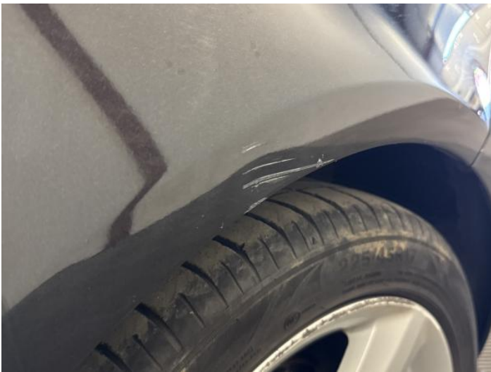
17: Wing osf Scratched Over 25mm Thru Paint
