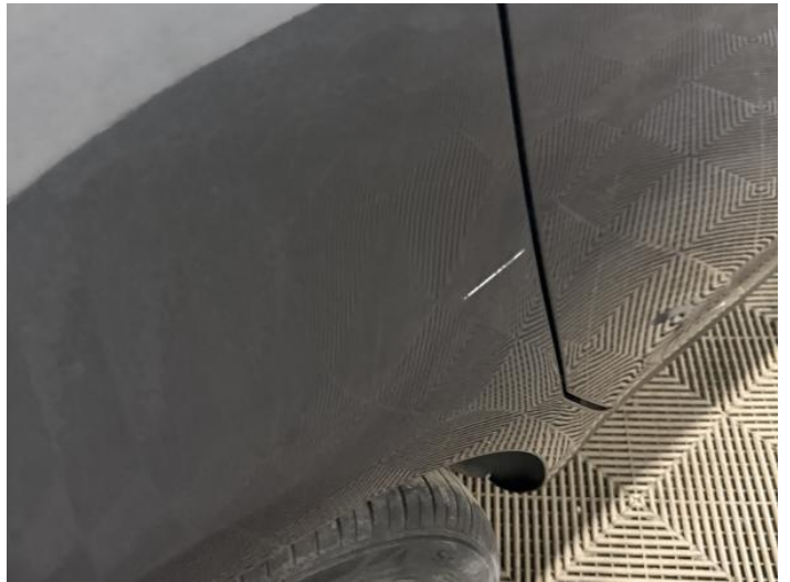
12: Qtr Panel osr Scratched Over 25mm Thru Paint
