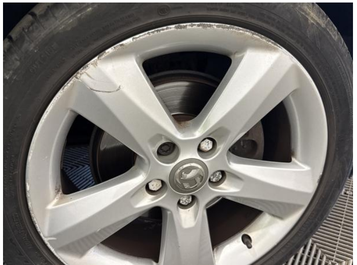
18: Wheel osf Scratched Over 50mm
