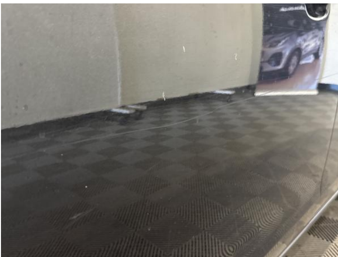
7: Door nsf Scratched Over 25mm Thru Paint
