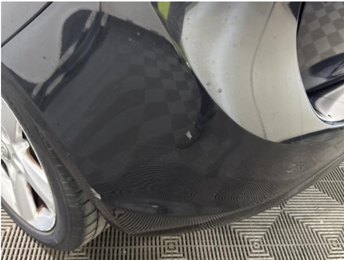
11: Bumper Rear Scratched 25 to 100mm Thru Paint
