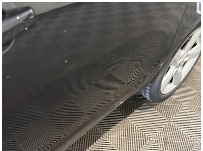
8: Door nsr Scratched Over 25mm Thru Paint
