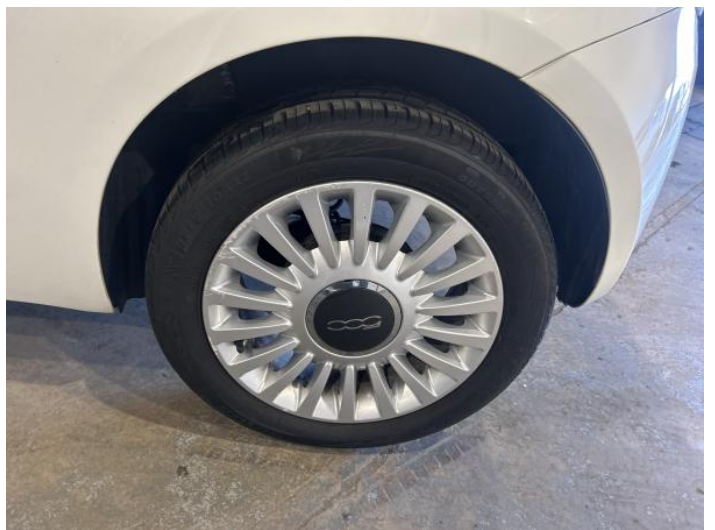
8: Wheel nsr Scratched Over 50mm
