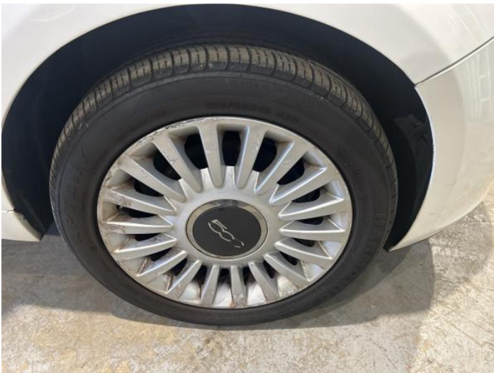
1: Wheel osf Scratched Over 50mm
