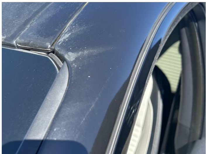
8: A Post ns Poor Previous Repair Poor Paint
