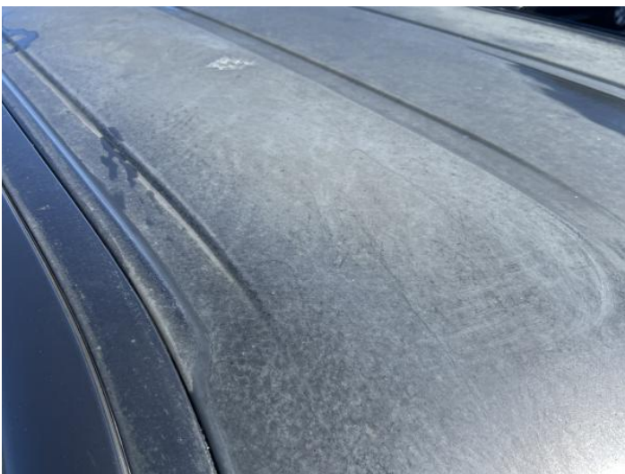
7: Roof Poor Previous Repair Poor Paint
