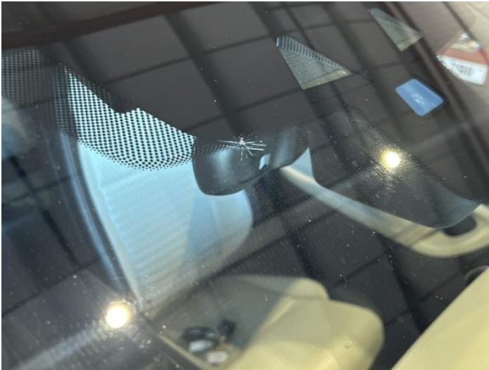
9: Screen Front Chipped Over 10mm
