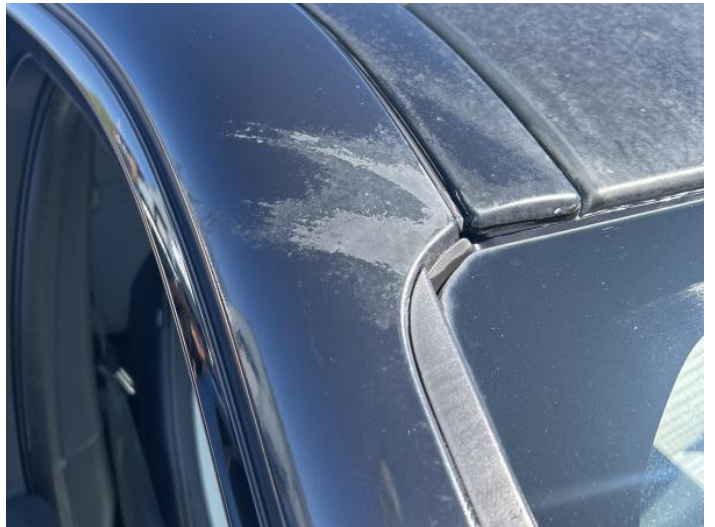
6: A Post os Poor Previous Repair Poor Paint
