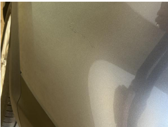
7: Bumper Rear Scratched 25 to 100mm Thru Paint
