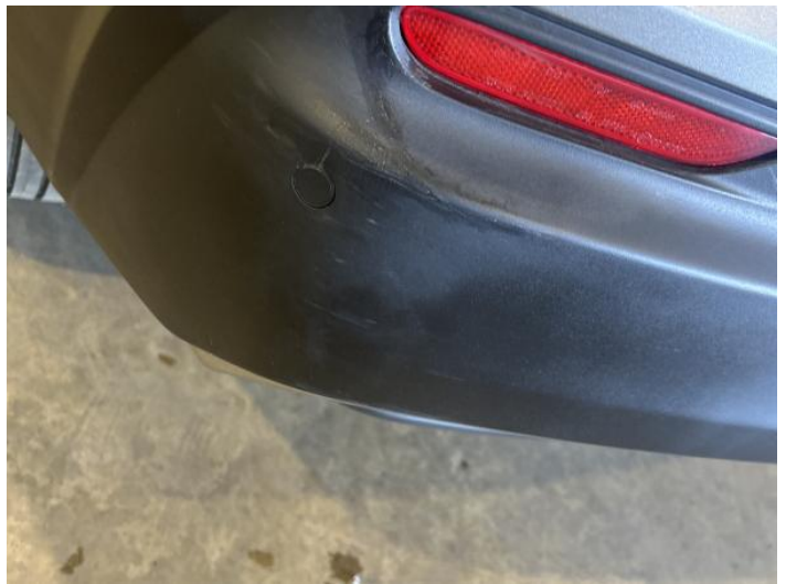
18: Bumper Rear Moulding Scuffed (Unpainted) UpTo 100mm
