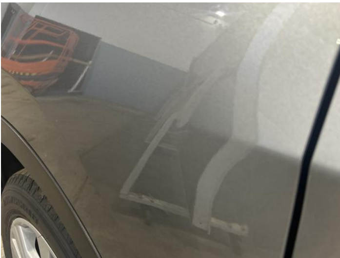
11: Wing nsf Dented 2 Or Less UpTo 10mm
