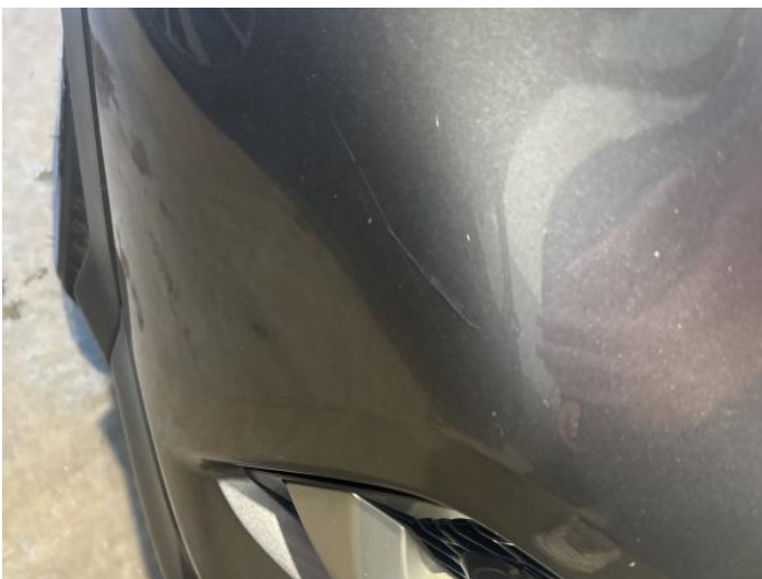
13: Bumper Front Scratched UpTo 25mm Thru Paint
