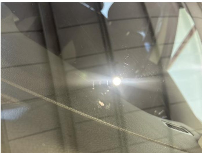
19: Screen Front Chipped UpTo 10mm
