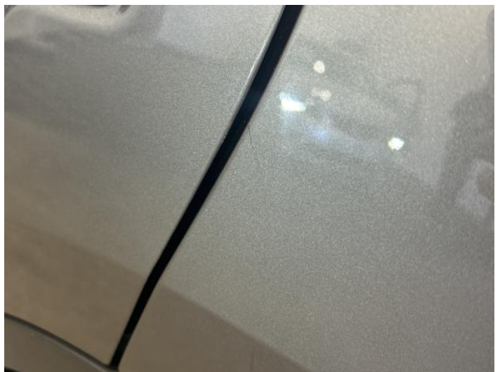
20: Qtr Panel nsr Scratched UpTo 25mm Thru Paint
