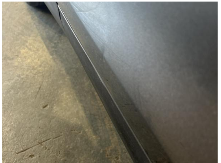
2: Door osf Dented Between 10mm + 30mm
