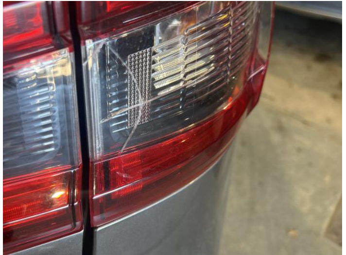
16: Lamp osr Broken Replace
