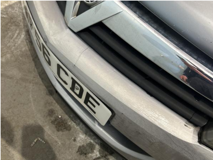
15: Bumper Front Cracked Over 25mm
