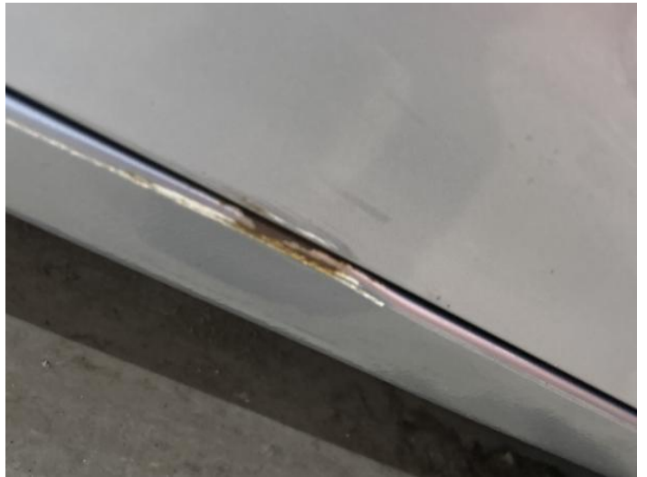
6: Door osf Scratched UpTo 25mm Thru Paint
