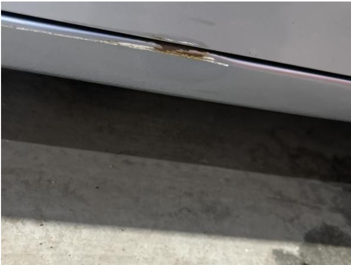
5: Sill os Dented With Paint Damage
