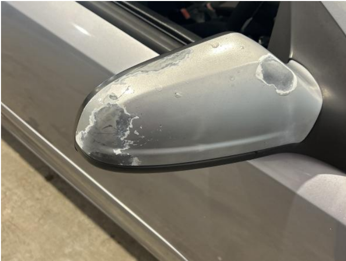
3: Door Mirror Assy osf Scratched (Painted) Over 25mm Thru Paint
