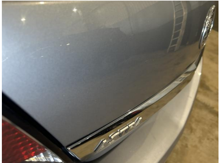
10: Tailgate Dented Between 10mm + 30mm
