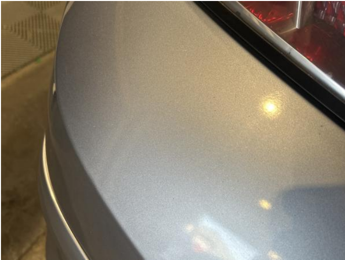
9: Bumper Rear Poor Previous Repair Poor Paint
