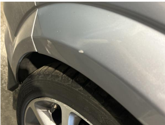
13: Wing nsf Dented With Paint Damage
