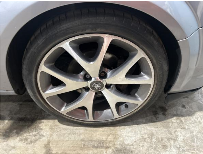
1: Wheel osf Scratched Over 50mm
