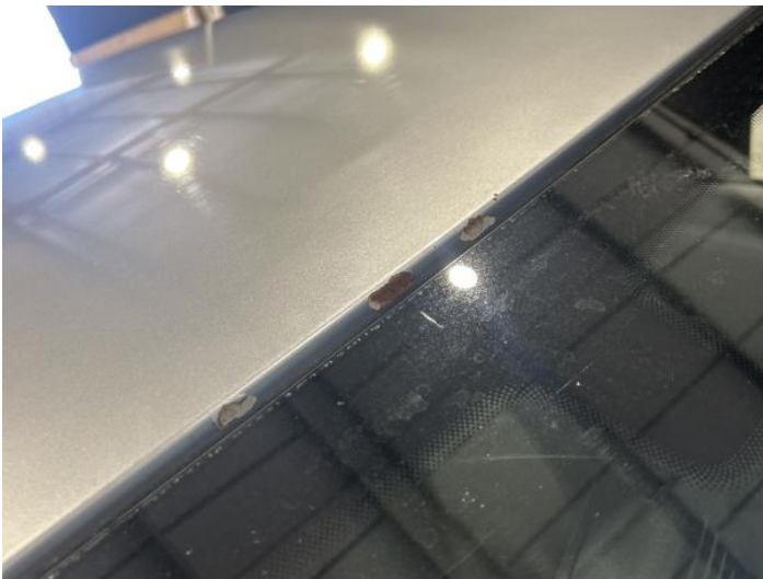
17: Roof Dented With Paint Damage
