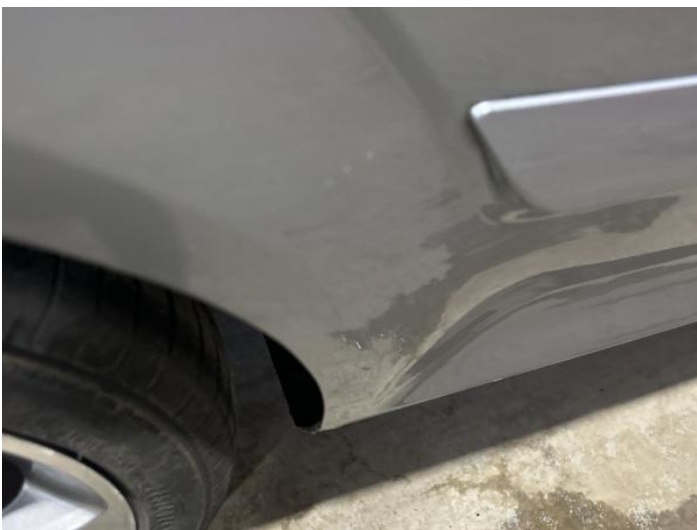
7: Qtr Panel osr Chipped 1 To 5
