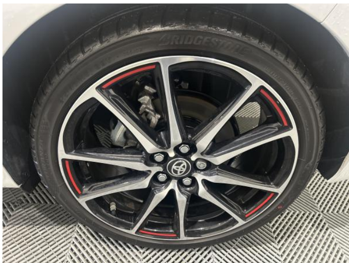
1: Wheel nsr Scratched Up To 50mm
