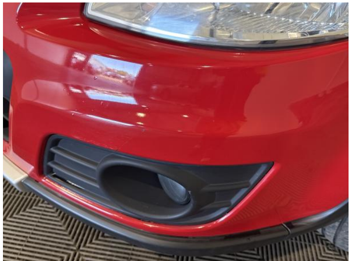
2: Bumper Front Scratched 25 to 100mm Thru Paint
