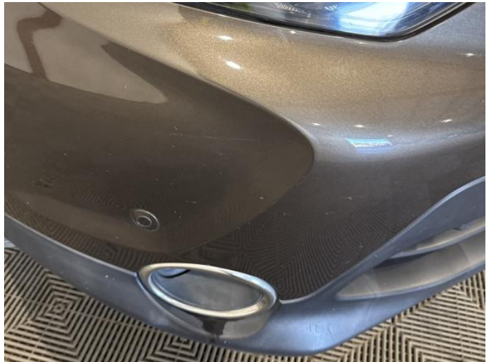
2: Bumper Front Scratched 25 to 100mm Thru Paint
