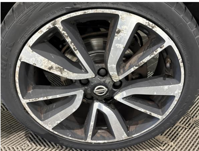
7: Wheel nsr Scratched Over 50mm
