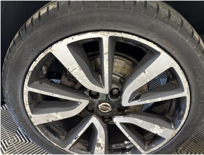
3: Wheel nsf Scratched Over 50mm
