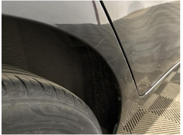
10: Qtr Panel osr Dented With Paint Damage
