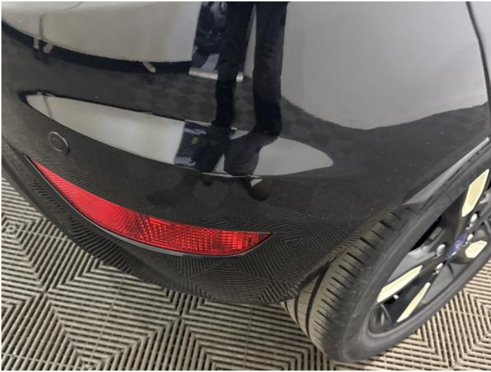
9: Bumper Rear Scratched 25 to 100mm Thru Paint
