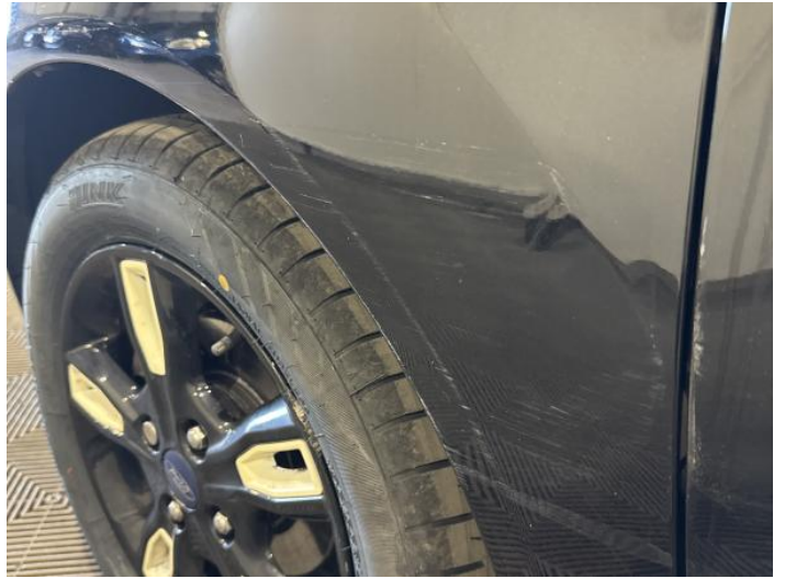
4: Wing nsf Dented With Paint Damage
