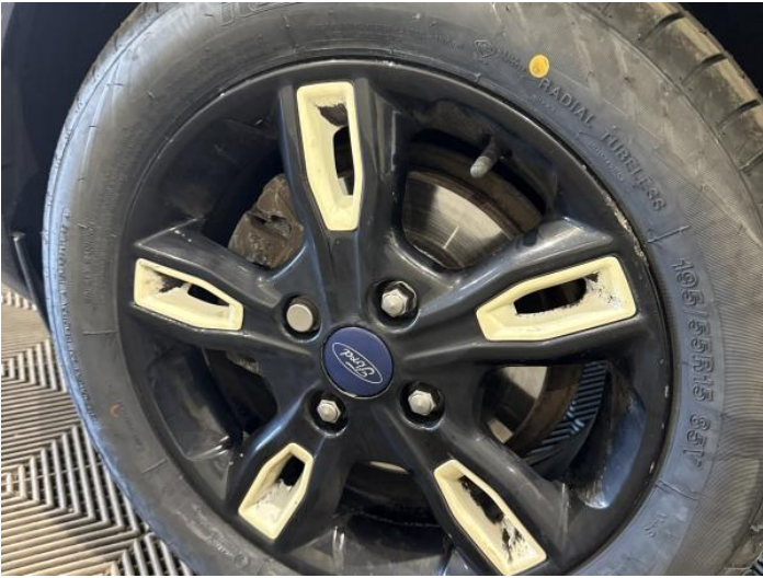
3: Wheel nsf Scratched Over 50mm
