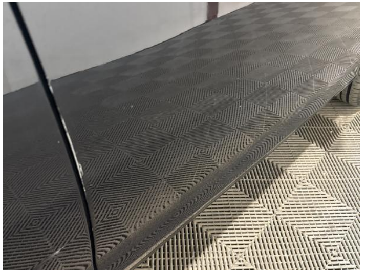
12: Door osf Scratched Over 25mm Thru Paint
