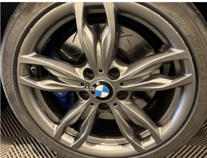
7: Wheel nsr Scratched Over 50mm
