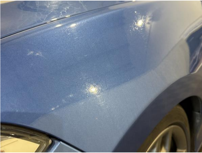
3: Wing nsf Poor Previous Repair Poor Paint
