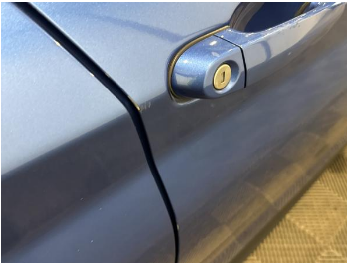
11: Door osf Chipped Edge Chip
