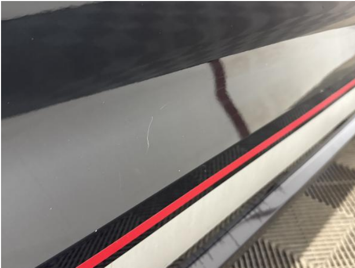
9: Door osf Scratched Over 25mm Thru Paint
