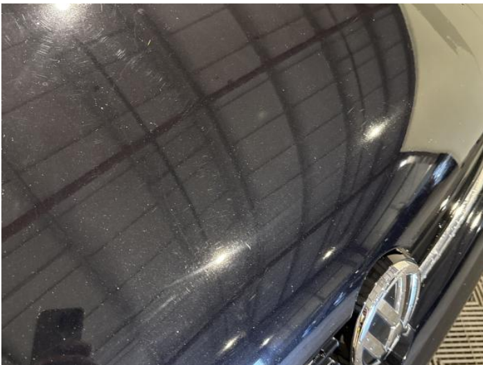
1: Bonnet Chipped Multiple Chips
