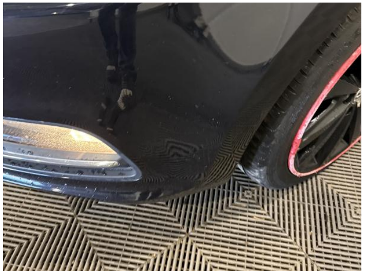
2: Bumper Front Chipped Multiple Chips
