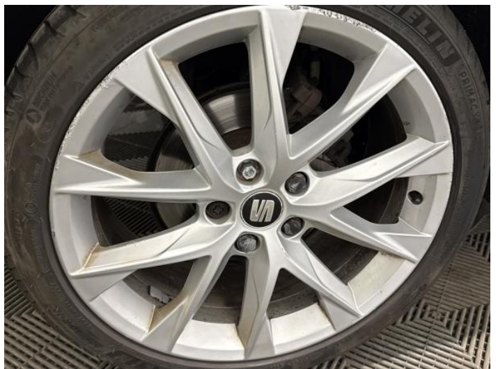
14: Wheel osr Scratched Over 50mm
