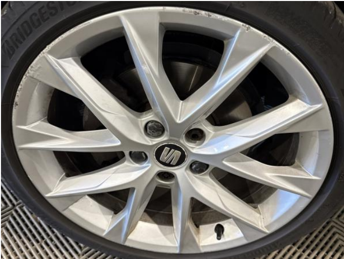
3: Wheel nsf Scratched Over 50mm
