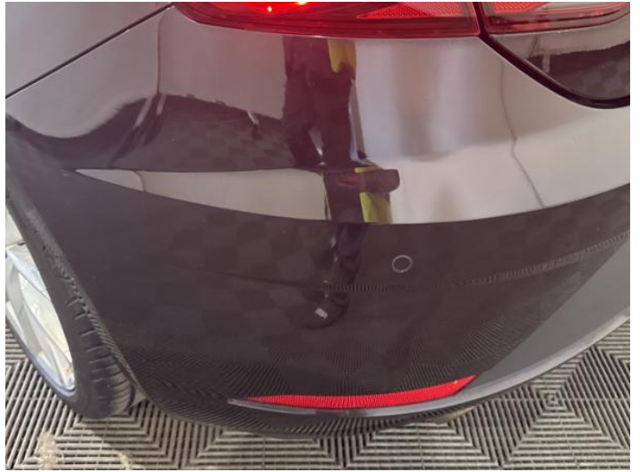
10: Bumper Rear Scratched 25 to 100mm Thru Paint
