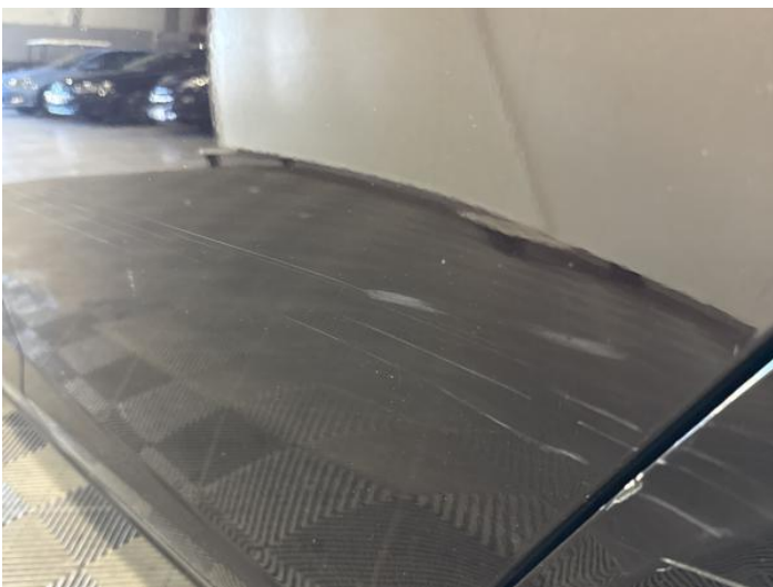
7: Door nsf Scratched Over 25mm Thru Paint
