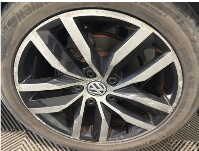
7: Wheel nsr Scratched Over 50mm
