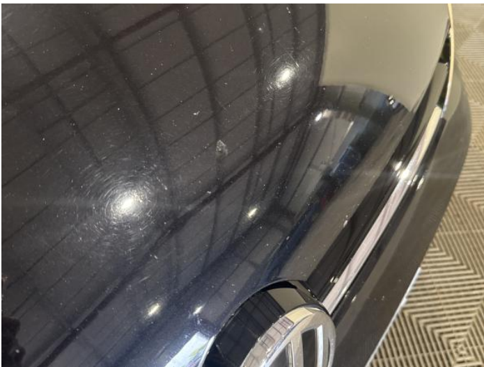
1: Bonnet Chipped Multiple Chips
