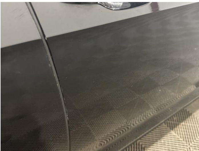
13: Door osf Chipped Edge Chip
