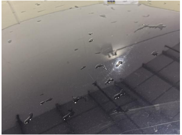
16: Roof Scratched Over 25mm Thru Paint
