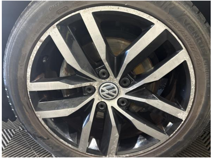
4: Wheel nsf Scratched Over 50mm
