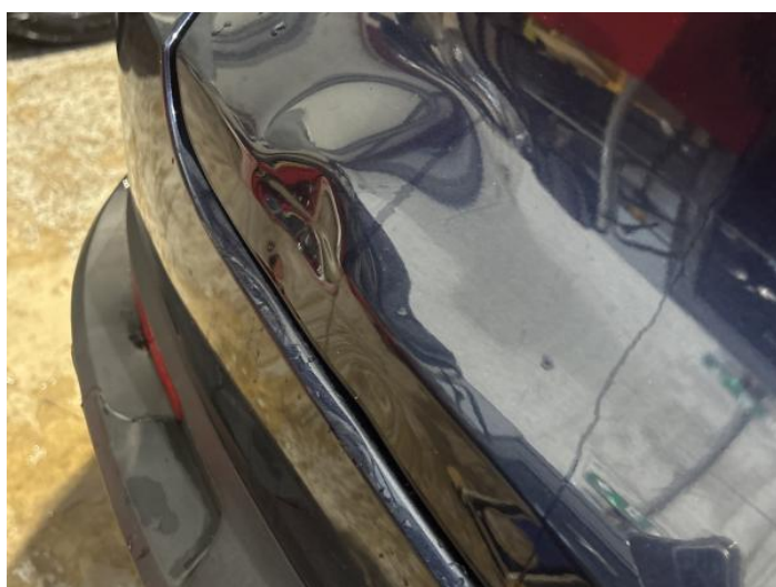
8: Tailgate Dented Over 30mm
