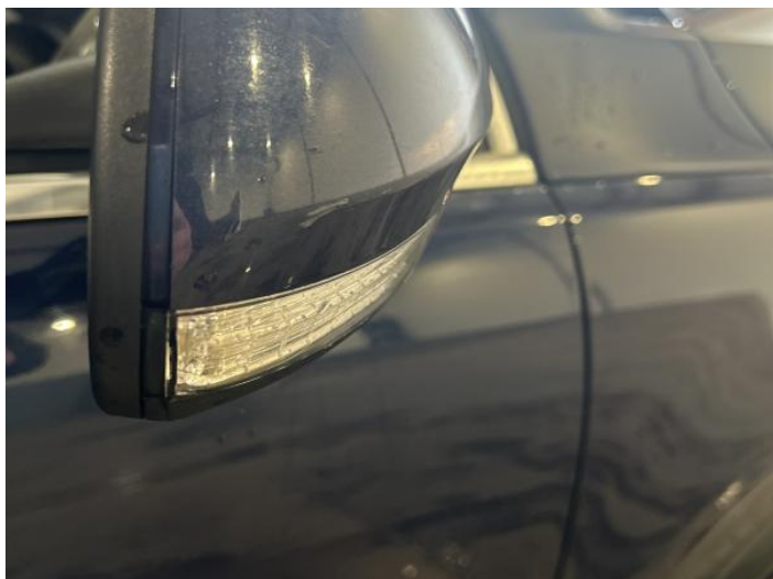
3: Door Mirror Assy osf Scratched (Painted) UpTo 25mm Not Thru Paint
