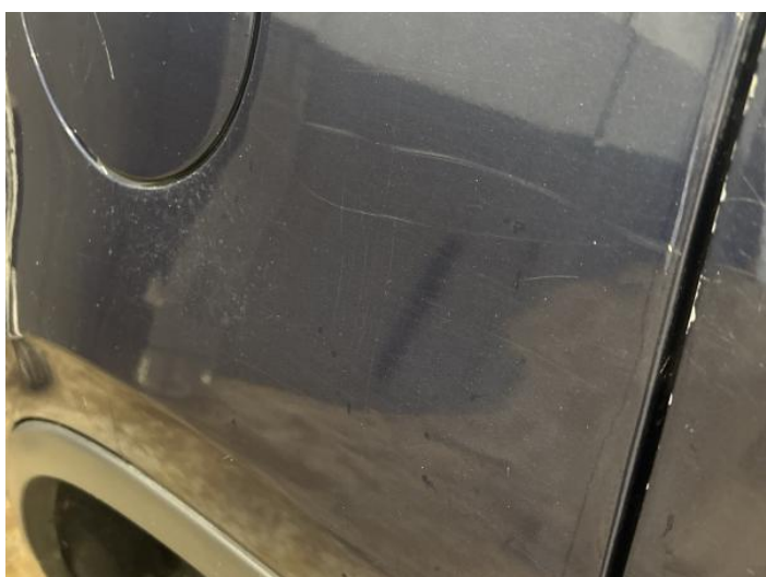
7: Qtr Panel osr Scratched Over 25mm Not Thru Paint
