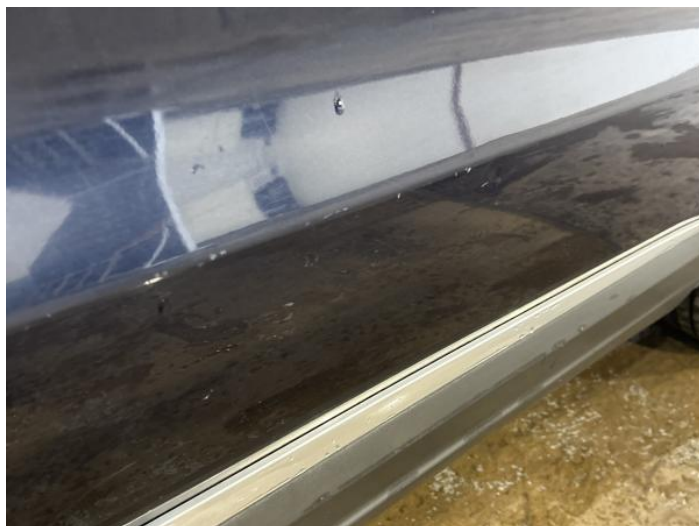
4: Door osf Chipped Multiple Chips
