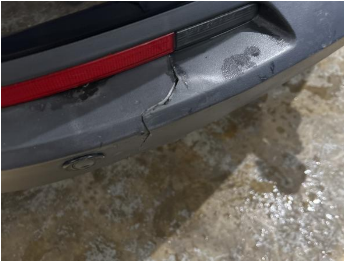
9: Bumper Rear Moulding Broken Replace
