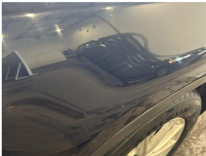
2: Wing of Scratched Over 25mm Not Thru Paint
