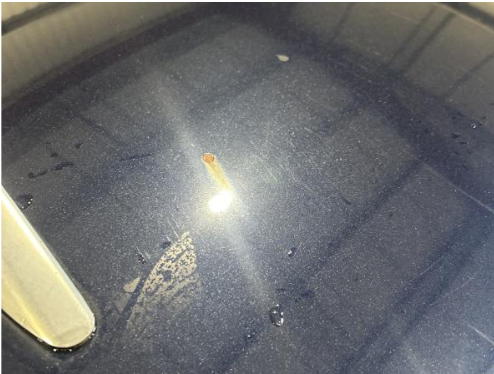
17: Roof Chipped 1 To 5
