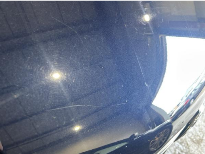
16: Bonnet Scratched Over 25mm Thru Paint
