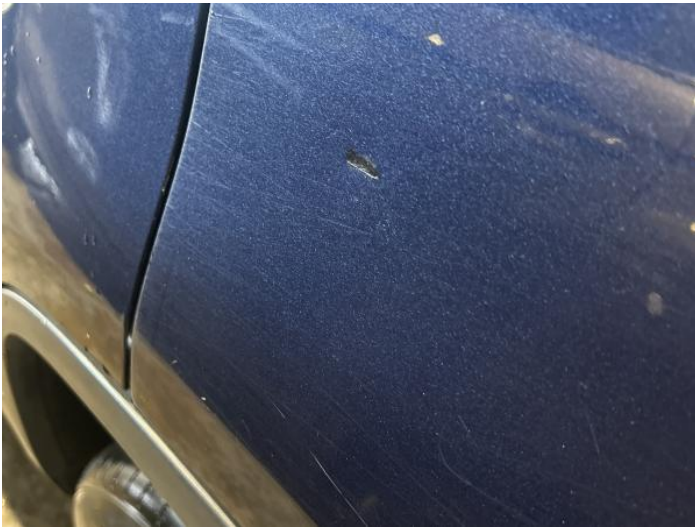
11: Qtr Panel nsf Dented With Paint Damage
