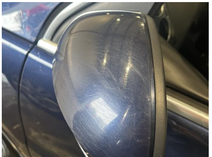
14: Door Mirror Assy nsf Scratched (Painted) Over 25mm Not Thru Paint
