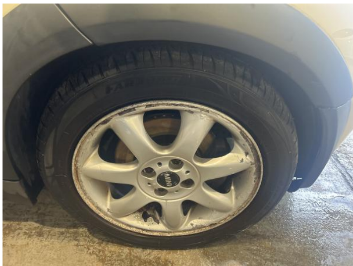
1: Wheel osf Corroded Light
