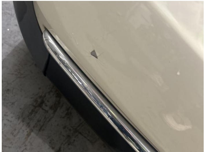
6: Bumper Rear Poor Previous Repair Paint Flake
