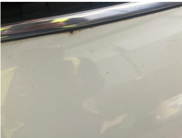
7: Tailgate Rusted UpTo 5mm
