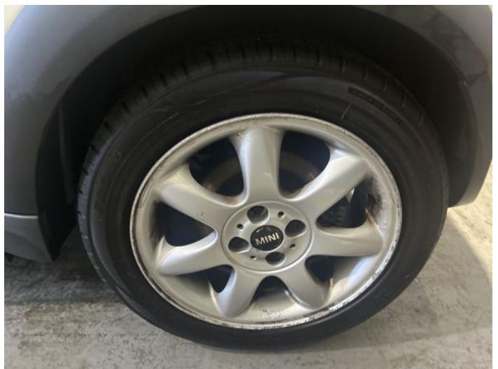
8: Wheel nsr Corroded Light
