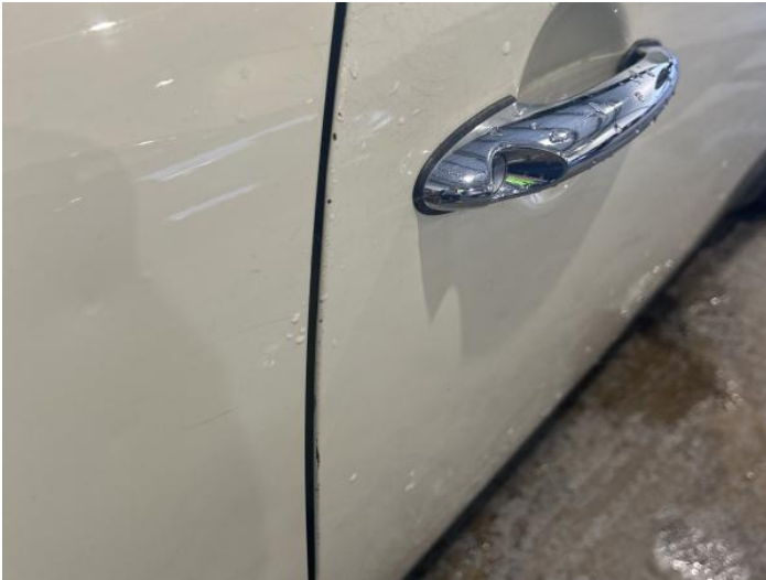
3: Door osf Chipped Edge Chip
