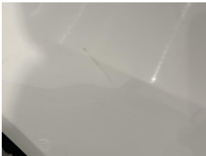
12: Wing nsf Scratched Over 25mm Thru Paint
