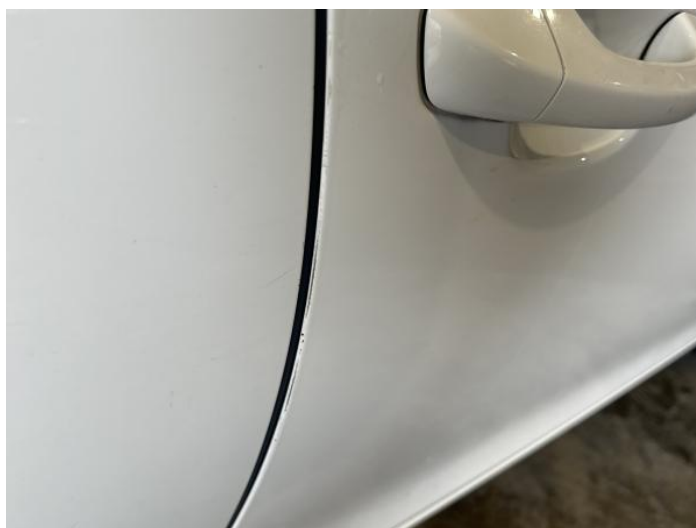
2: Door osf Chipped Edge Chip
