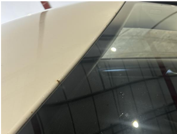
17: Roof Chipped Edge Chip
