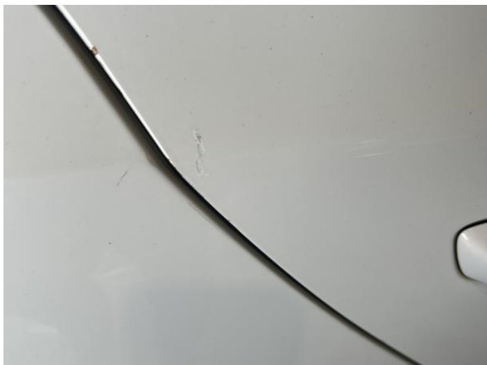
3: Door osr Scratched UpTo 25mm Thru Paint
