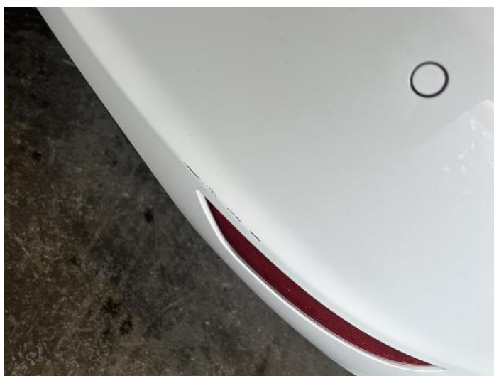
6: Bumper Rear Scratched 25 to 100mm Thru Paint
