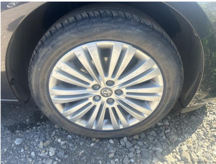
1: Wheel osf Scratched Over 50mm
